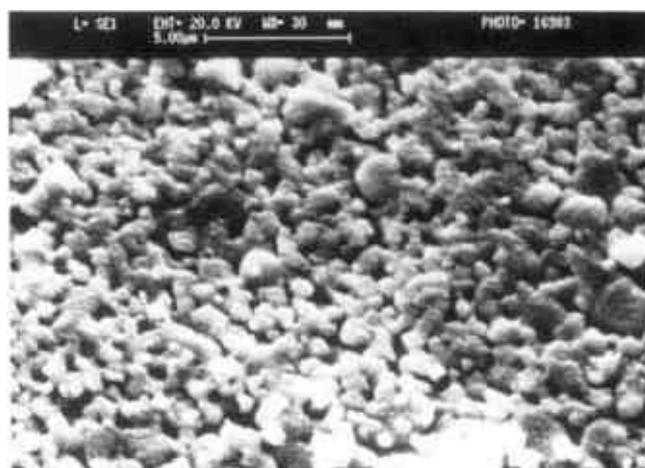
**Figure 5.** Scanning electron micrograph of  $\text{MgTa}_2\text{O}_6$ .
