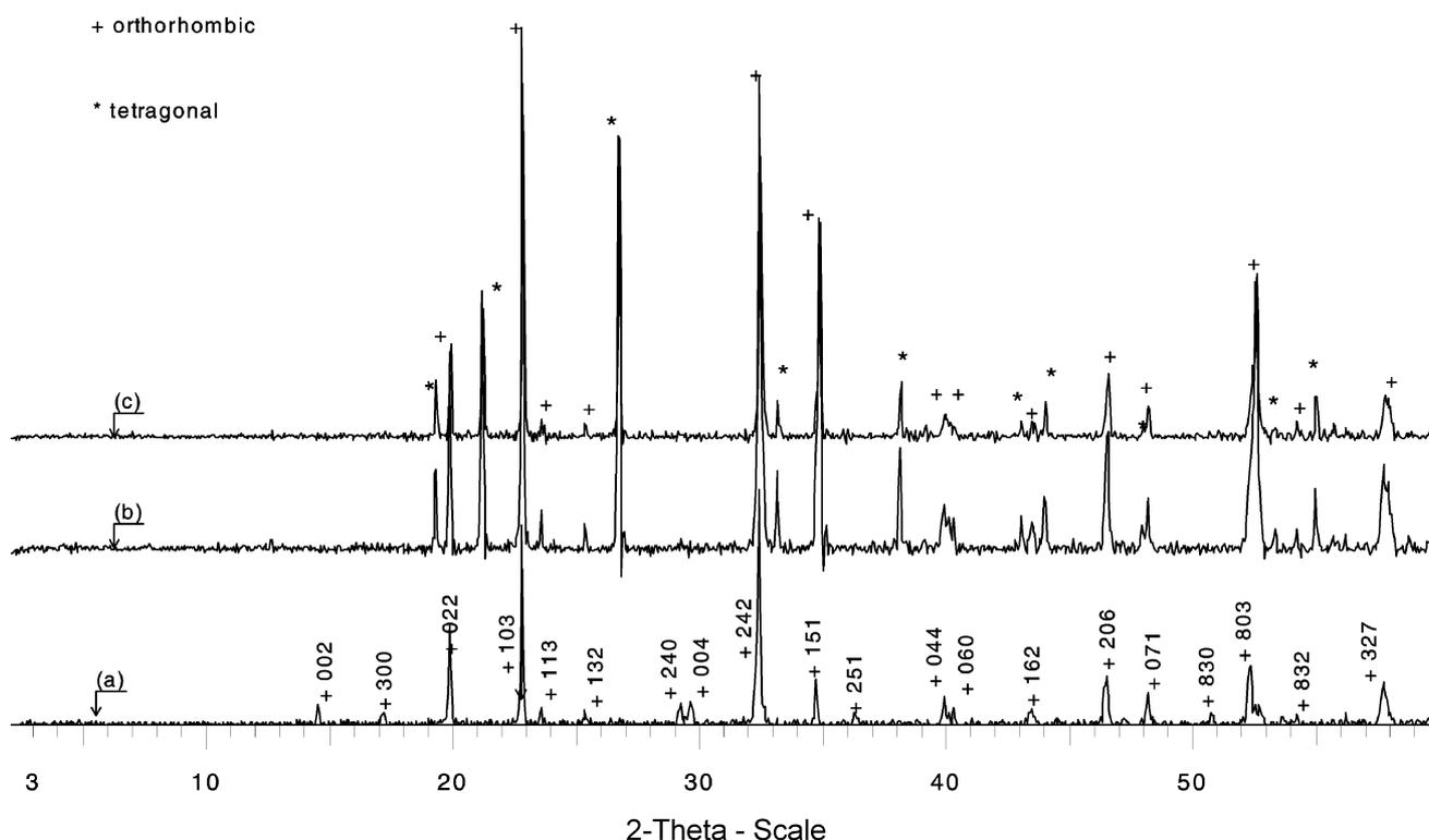
**Figure 1.** Powder X-ray diffraction pattern of MgTa<sub>2</sub>O<sub>6</sub> heated at (a) 850°C for 6 hours, (b) 1100°C for 16 hours and (c) 1200°C for 12 hours.
