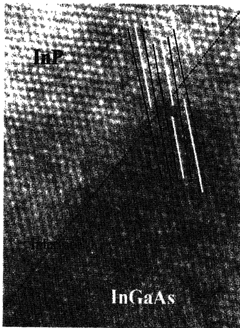
Figure 6. HRTEM of InGaAs/InP interface showing the presence of dipoles.
