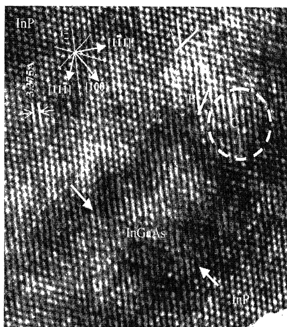
Figure 5. HRTEM of InGaAs well showing different planes and defects.
