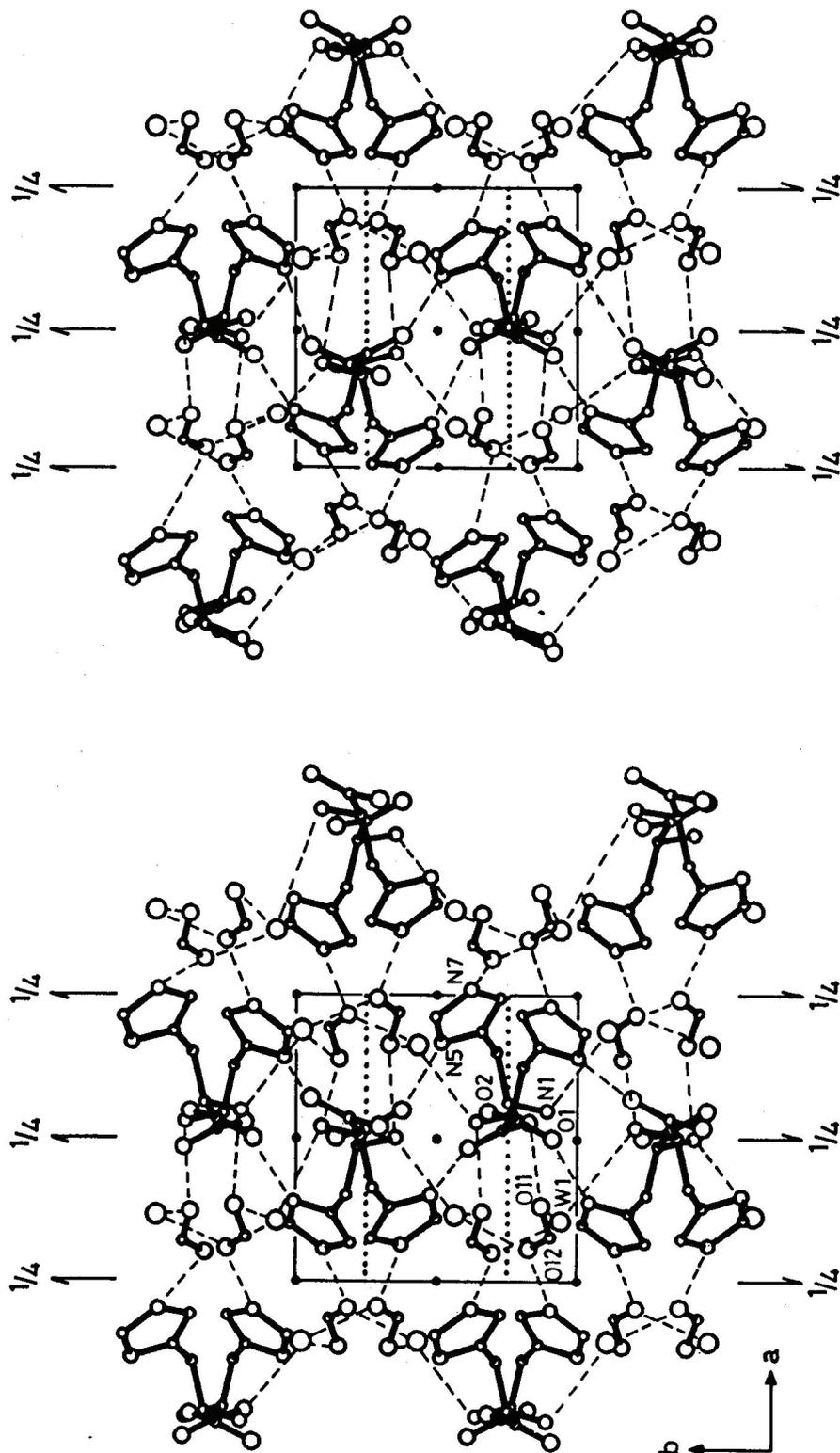
Figure 2. Crystal structure of DL-histidine formate monohydrate. Only nitrogen and oxygen atoms are numbered. The hydrogen bond between N1 of one molecule and O2 of a glide related molecule has not been shown, as the atoms partially overlap.
