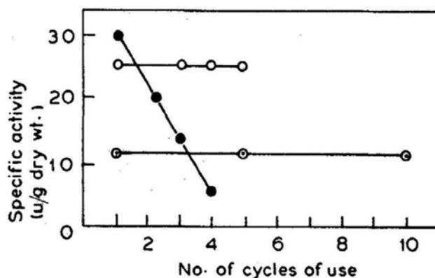
**Figure 2.** Operational stability of *K. citrophila* penicillin acylase immobilized by covalent attachment to silanized controlled-pore ceramics.
