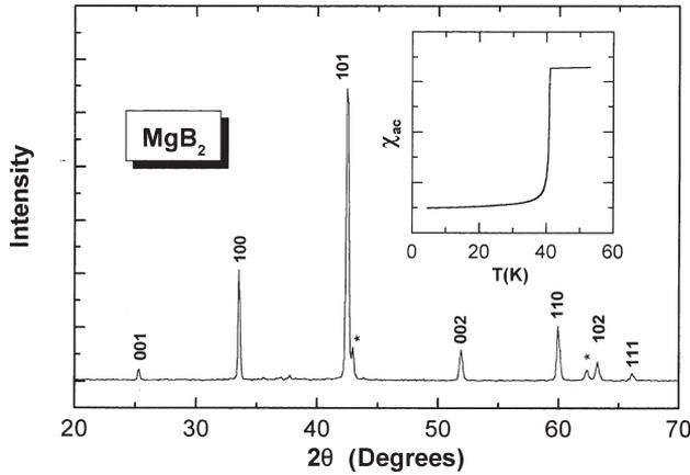
**Figure 1.** X-ray diffraction pattern of  $\text{MgB}_2$  indexed to hexagonal  $P6/mmm$  structure. The impurity lines due to  $\text{MgO}$  are indicated by asterisks. The inset shows the superconducting transition at 39.4 K.
