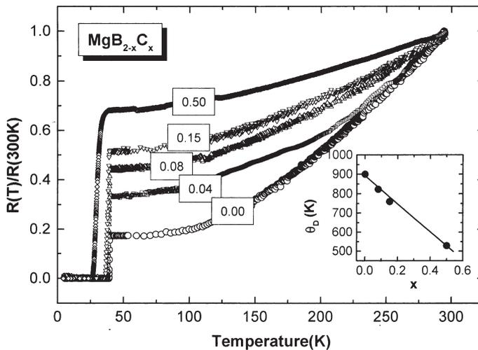
**Figure 4.** Superconducting transition in MgB<sub>2-x</sub>C<sub>x</sub> as seen in resistivity measurements. The resistivity in the normal state has been fitted to Bloch–Gruneisen expression. The inset shows the variation of Debye temperature,  $\theta_D$  with carbon content.
