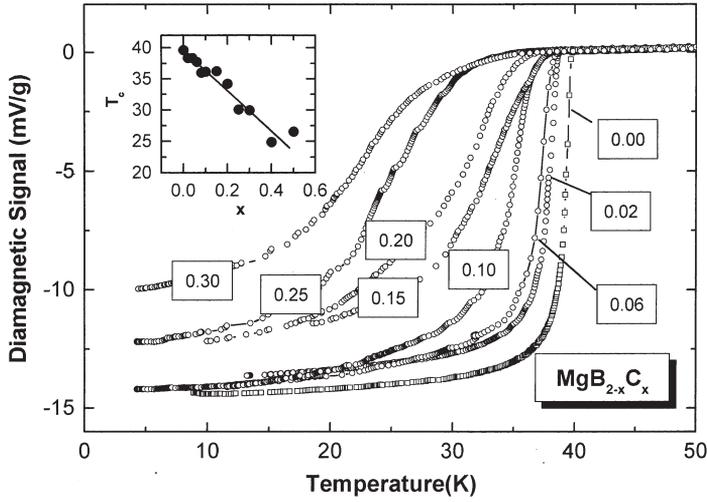
**Figure 2.** Susceptibility measurements indicating the superconducting transition in  $\text{MgB}_{2-x}\text{C}_x$ . The inset shows the variation of  $T_c$  with carbon content  $x$ .
