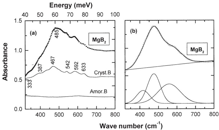
**Figure 6.** (a) Absorption spectrum of  $MgB_2$ . Also shown are the absorption spectra of the starting crystalline and amorphous B. (b) Fits of the absorption spectrum at 297 K in terms of sum of three Gaussians and a linear background.
