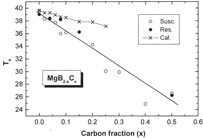
**Figure 5.** Variation of  $T_c$  with carbon content in  $MgB_{2-x}C_x$ , as obtained from susceptibility and resistivity measurements. The dashed line indicates the expected decrease in  $T_c$  due to volume change (see text).
