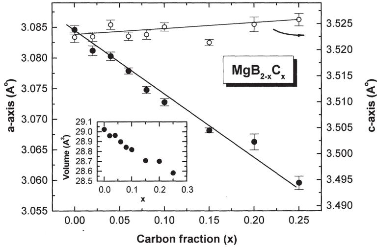
**Figure 3.** Variation of lattice parameters with carbon content in MgB<sub>2-x</sub>C<sub>x</sub>. The inset shows the variation of lattice volume with carbon concentration.
