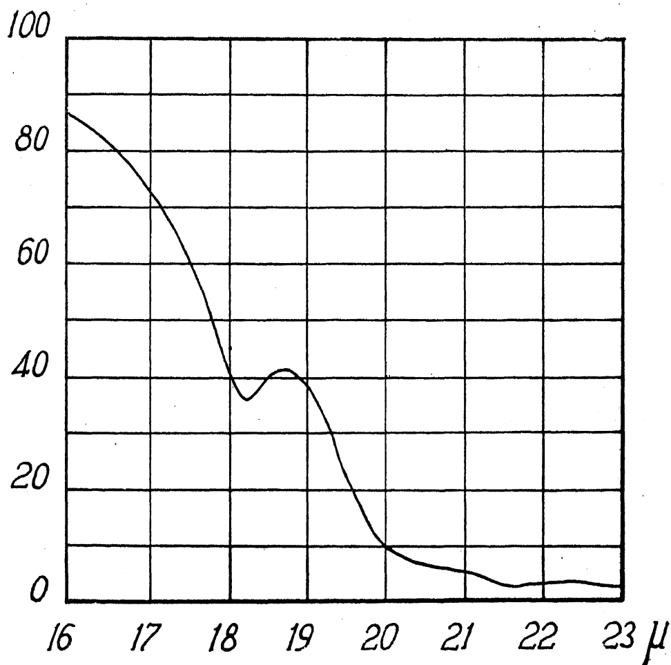
FIG. 12. Absorption by NaF; plate thickness: 0.18 mm.
