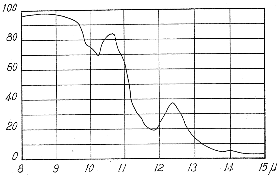
FIG. 7. Transmission by an MgO plate 0.06 mm. thick.
