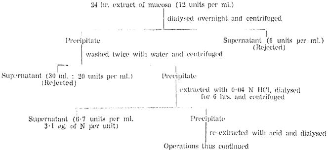
By continuing the above series of operations, enzyme preparations at as low a level as 1-4  $\mu g$ , of N per unit have been obtained.
