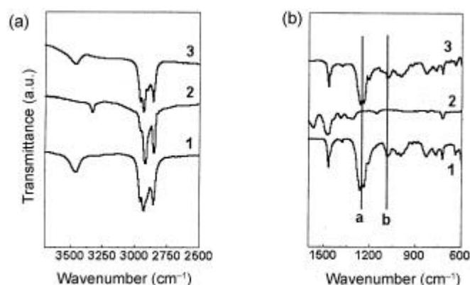
**Figure 3.** (a) and (b) FTIR spectra of pure SDS (curve 1), ODA-capped gold nanoparticles (curve 2) and surface modified gold nanoparticles with interdigitated bilayers of ODA and SDS (curve 3) in different spectral windows.
