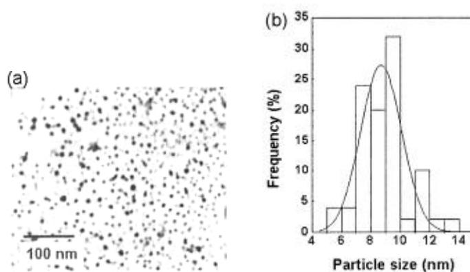
**Figure 4.** (a) Representative TEM micrograph of a film of gold nanoparticles phase transferred into water (SDS-ODA-Au). (b) Histogram showing the particles' size distribution measured from figure 4a. The solid line represents a Gaussian fit to the data.
