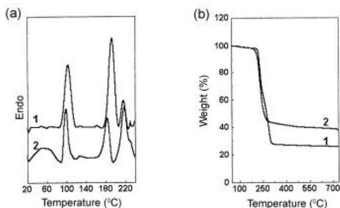
**Figure 2.** (a) DSC data recorded from powders of pure SDS (curve 1) and ODA-capped gold nanoparticles after phase transfer into water (curve 2). The curves have been shifted vertically for clarity. (b) TGA data recorded for powders of pure SDS (curve 1) and ODA-capped gold nanoparticles after phase transfer into water (curve 2).
