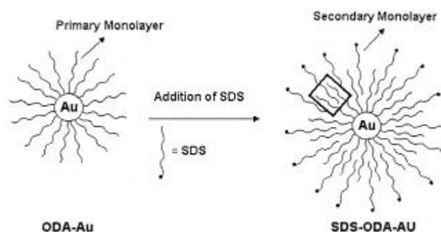
**Scheme 1.** Diagram showing the formation of an interdigitated secondary monolayer of SDS molecules on the surface of ODA-modified gold particles (SDS-ODA-Au). The box encloses ordered, interdigitated regions of the bilayers (see text for details).
