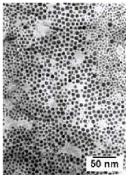
Figure 5. TEM micrograph of gold nanoparticles phase transferred into toluene self-assembled by solvent evaporation.
