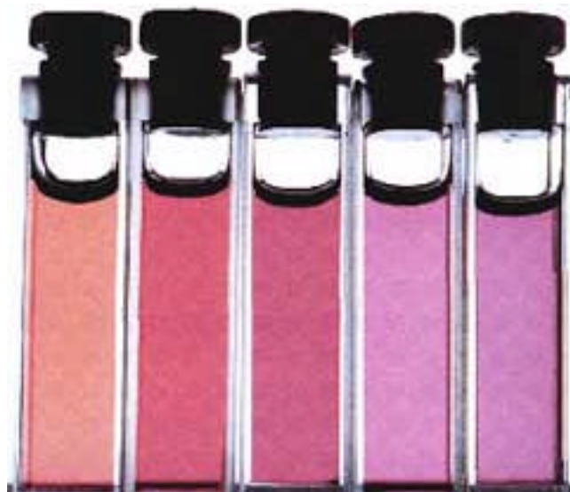
Figure 1. Five sols of colloidal gold prepared in water and in mixtures of butyl acetate and CS 2 . Refractive indices of the solutions at the absorption band maximum are 1.336, 1.407, 1.481, 1.525 and 1.583 ( \pm 0.004 ) respectively. (Reprinted with permission from ref. 49, © 1994, American Chemical Society.)
