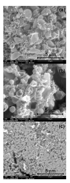
**Figure 2.** SEM microstructure of silica films synthesized at heptane–water interface using 1 M NH<sub>4</sub>OH subphase: (a) without any surfactant in the sub-phase, (b) 1 CMC CTAB sub-phase and (c) 1 CMC SDS sub-phase (scale bar represents 5  $\mu$ m).
