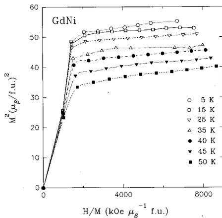
FIG. 4. Arrott plots for GdNi. The lines drawn through the data points are guides to the eye.
