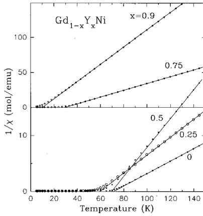
FIG. 1. Inverse susceptibility as a function of temperature (2–150 K) for the alloys,  $\text{Gd}_{1-x}\text{Y}_x\text{Ni}$ . The continuous lines represent the least-squares fit of the data to Curie-Weiss behavior in the paramagnetic state.
