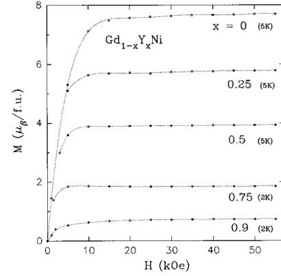
FIG. 2. Isothermal magnetization behavior of the alloys,  $\text{Gd}_{1-x}\text{Y}_x\text{Ni}$  ( $x=0.0, 0.25, 0.5, 0.75, 0.9$ ). A smooth line is drawn through the data points.
