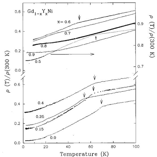
FIG. 6. Electrical resistivity as a function of temperature below 100 K for the alloys,  $\text{Gd}_{1-x}\text{Y}_x\text{Ni}$  ( $x=0.0, 0.15, 0.25, 0.4, 0.5, 0.6, 0.7, 0.8,$  and  $0.9$ ). The arrows indicate the values of  $T_C$  as mentioned in Table I.
