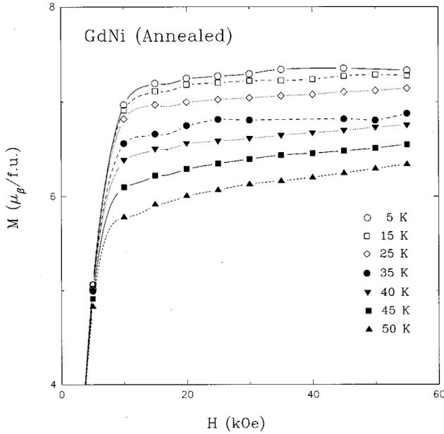
FIG. 3. Isothermal magnetization at several temperatures for the annealed specimen of GdNi. A line drawn through the data points for each temperature serves as a guide to the eyes.
