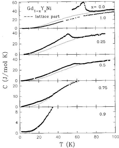
FIG. 7. Heat-capacity ( $C$ ) as a function of temperature in the alloys,  $\text{Gd}_{1-x}\text{Y}_x\text{Ni}$  ( $x=0.0, 0.25, 0.5, 0.75, 0.9$ , and  $1.0$ ). The lattice part is obtained as described in Ref. 17.
