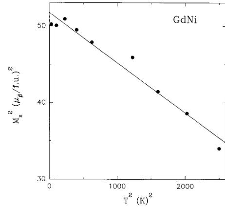
FIG. 5. Square of spontaneous magnetization as a function of square of temperature for GdNi. The continuous line is a linear fit to the data points.
