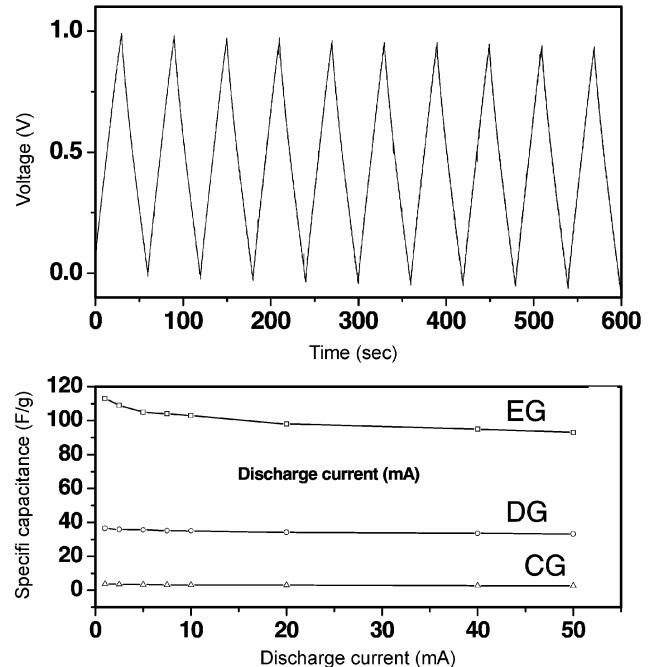
**Figure 3.** (a) Typical charging and discharging curves of EG at 5 mA and (b) specific capacitance as a function of discharge current.
