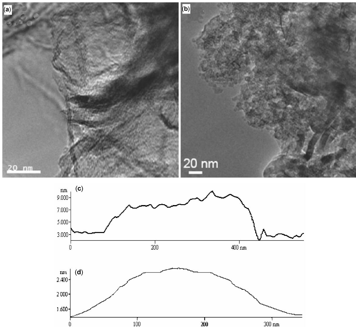
**Figure 1.** TEM images of (a) graphene obtained by the thermal exfoliation of graphitic oxide (EG). (b) thermal conversion of nanodiamond to graphene (DG). (c) and (d) AFM height profiles of EG and DG respectively.
