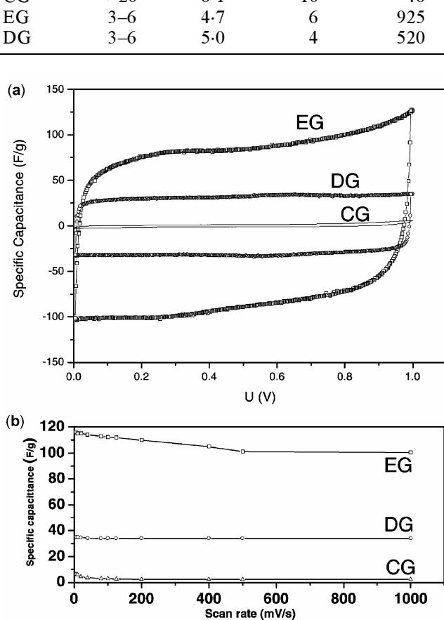
**Figure 2.** (a) Voltammetry characteristics of a capacitor built from graphene electrodes (5 mg each) at a scan rate of 100 mV/s using (a) aqueous H<sub>2</sub>SO<sub>4</sub> (1 M) and (b) specific capacitance as a function of scan rate.
