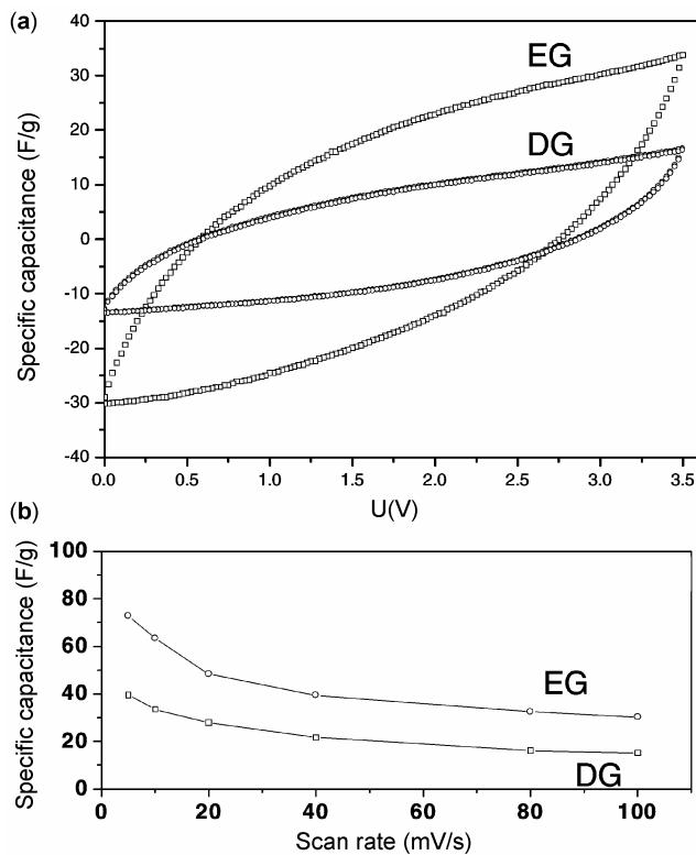
**Figure 5.** (a) Voltammetry characteristics of a capacitor built from graphene electrodes (5 mg each) at a scan rate of 100 mV/s using ionic liquid. (b) Specific capacitance as a function of scan rate using PYR<sub>14</sub>TFSI.
