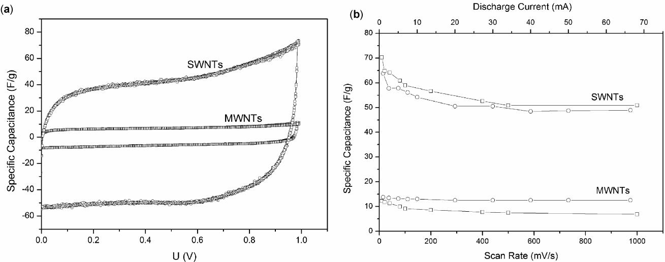
**Figure 4.** (a) Voltammetry characteristics of a capacitor built from SWNTs and MWNTs at a scan rate of 100 mV/s using 1 M  $\text{H}_2\text{SO}_4$ . (b) Specific capacitance of SWNTs and MWNTs as function of scan rate (open squares) and discharge current (open circles).
