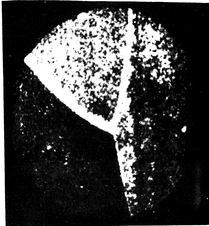
Figure 11. SIMS ion image showing carbon segregation to grain boundaries in NiSiCrCoMo steel.
