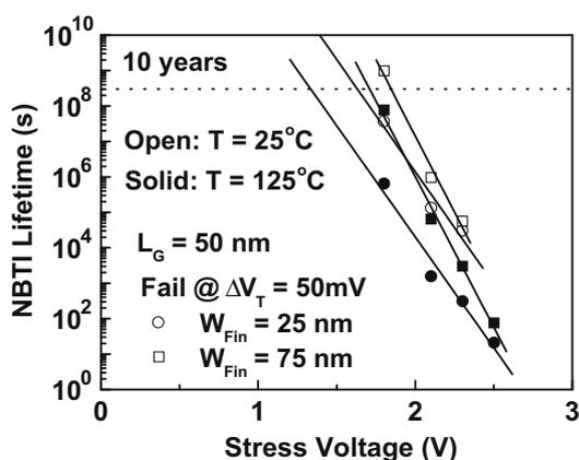
Fig. 13. Extracted NBTI lifetime as a function of stress voltage at  $25^\circ\text{C}$  and  $125^\circ\text{C}$  for different fin widths. Narrow fins show worse NBTI lifetime.
