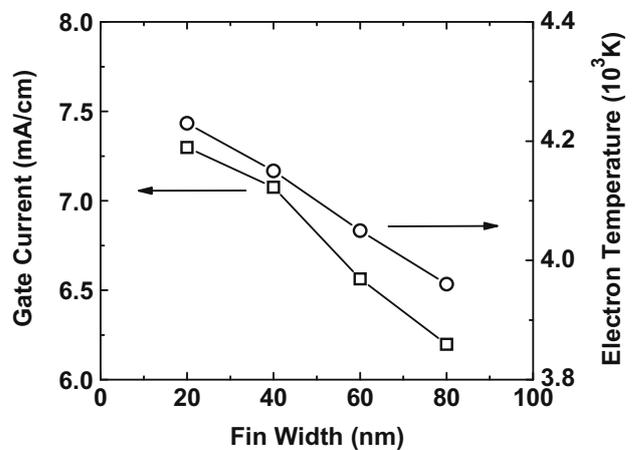
Fig. 11. Simulated gate current (left axis) and electron temperature (right axis) by 2D Medici device simulations. The simulated structures have a  $\text{SiO}_2$  gate oxide thickness of 1.9 nm, a body doping of  $10^{15} \text{ cm}^{-3}$ , a gate length of 50 nm and different fin widths ranging from 20 nm to 80 nm. For narrow fins the gate injection increases due to the higher electron temperature.
