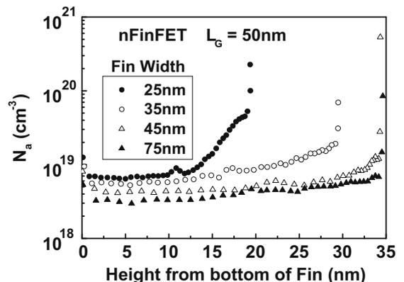
Fig. 7. Fin extension doping profile as a function of height from the bottom of fin for different fin widths. Doping profile shows significant variation along the height of the fin for narrower fins.
