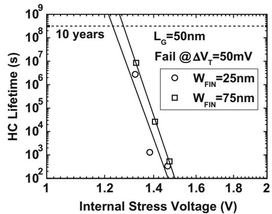
Fig. 10. Extracted lifetime for HC stress condition  $V_{Gint} = V_{Dint}$  as a function of stress voltage for different fin widths. Narrow fins show worse HC lifetime.
