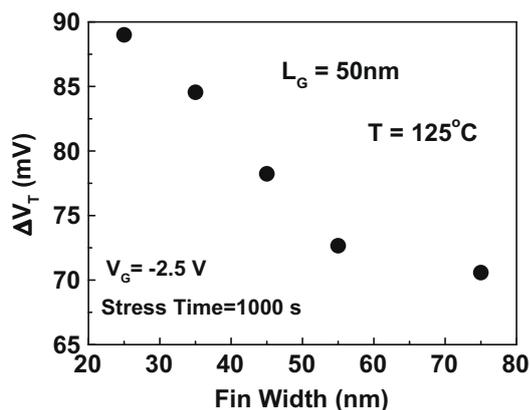
Fig. 12. Threshold voltage shift after stressing pFinFET at  $V_G = 2.5$  V,  $125^\circ\text{C}$  for 1000 s as a function of fin width.
