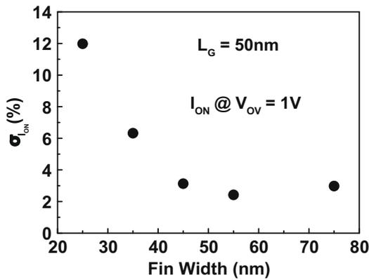
Fig. 8. Percentage standard deviation in ON current versus fin width for the devices with  $L_G = 50$  nm. ON current measured at  $V_{OV} = 1$  V and  $V_{DS} = 1.2$  V. Narrow fin shows higher  $I_{ON}$  variability due to non-uniformity in the extension region.
