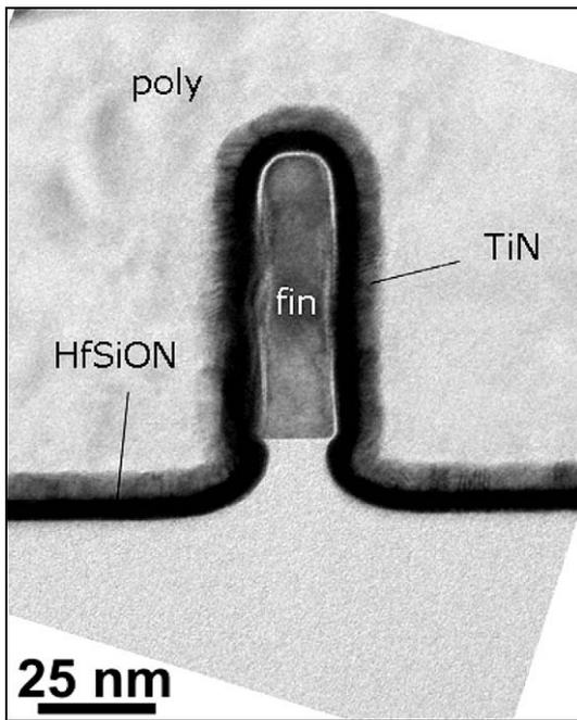
Fig. 1. A cross sectional TEM image of the fin after gate patterning.
