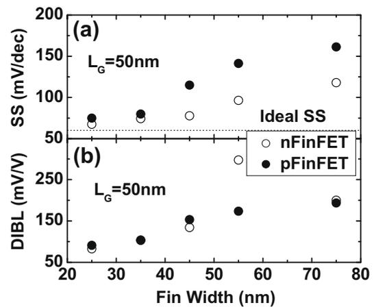
Fig. 3. (a) Sub-threshold swing and (b) DIBL as a function of fin width for nFinFET and pFinFET devices with  $L_G = 50\text{ nm}$ . Significant improvements are observed in narrow fins.
