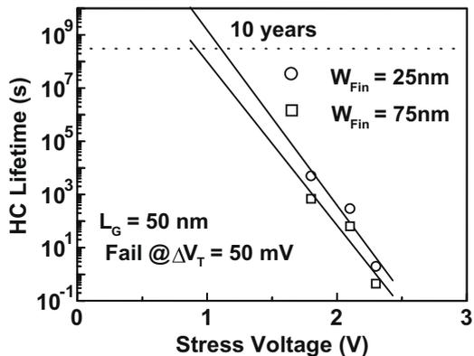
Fig. 9. Extracted lifetime for HC stress condition  $V_G = V_D$  as a function of stress voltage for different fin widths. Narrow fins show improved HC lifetime.
