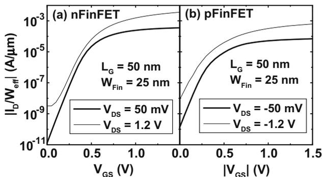
Fig. 2.  $I_D$ - $V_{GS}$  characteristics of nFinFETs and pFinFETs with  $L_G = 50\text{ nm}$  and  $W_{Fin} = 25\text{ nm}$  at low and high  $V_{DS}$ .  $I_D$  is normalized by effective fin width ( $W_{eff} = 2H + W_{Fin}$ ).
