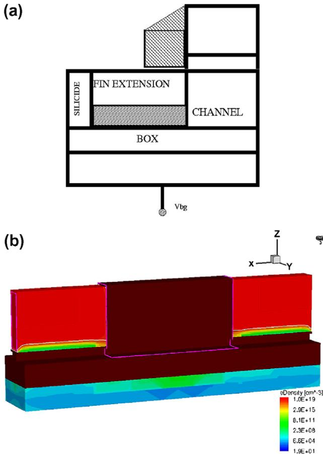
Fig. 6. (a) Cross section of one half of the FinFET (including extension region) showing the depletion of fin extension, due to back gate. (b) 3D perspective view of the carrier distribution in the FinFET structure at  $V_{BG} = -40$  V showing the depletion of carriers in the bottom of fin.
