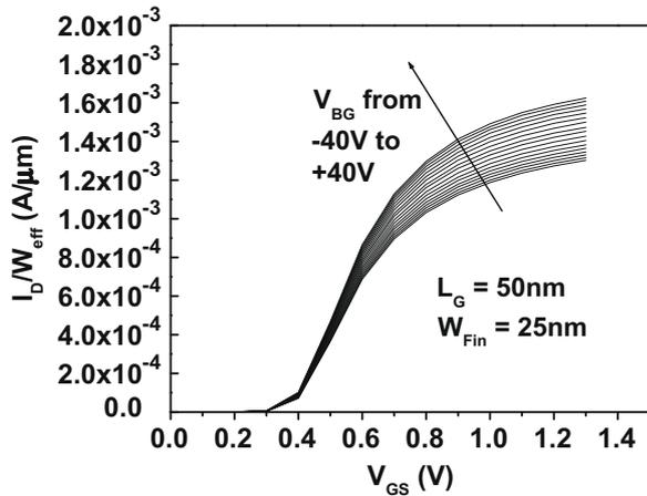
Fig. 5.  $I_D$ - $V_G$  measurement of nFinFET with  $L_G = 50$  nm,  $W_{Fin} = 25$  nm and  $H_{Fin} = 60$  nm, showing the sensitivity of  $I_{ON}$  on the back gate voltage ( $-40$  V to  $+40$  V) with  $t_{BOX} = 145$  nm.
