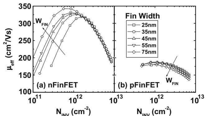
Fig. 4. Effective carrier mobilities as a function of inversion carrier density for different fin widths. Due to different mobility behaviours of electrons and holes in (1 0 0) and (1 1 0) planes, the overall carrier mobility decreases for narrow nFinFETs and slightly increases for narrow pFinFETs.
