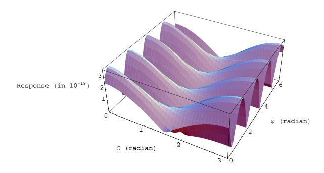
Figure 3: Response  $\mathcal{R}_M$  of LISA to the jet source at f=1 mHz as function of angular location  $(\theta, \phi)$  of the source for the Michelson combination.
