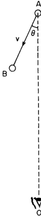
Figure 1. In the beam model schematically shown here A is the stationary component and B is the component beamed at the observer O. For apparent superluminal motion to manifest, the angle \theta has to be very small.
