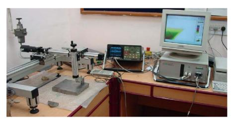
Figure 5: Experimental set up of SAFT
