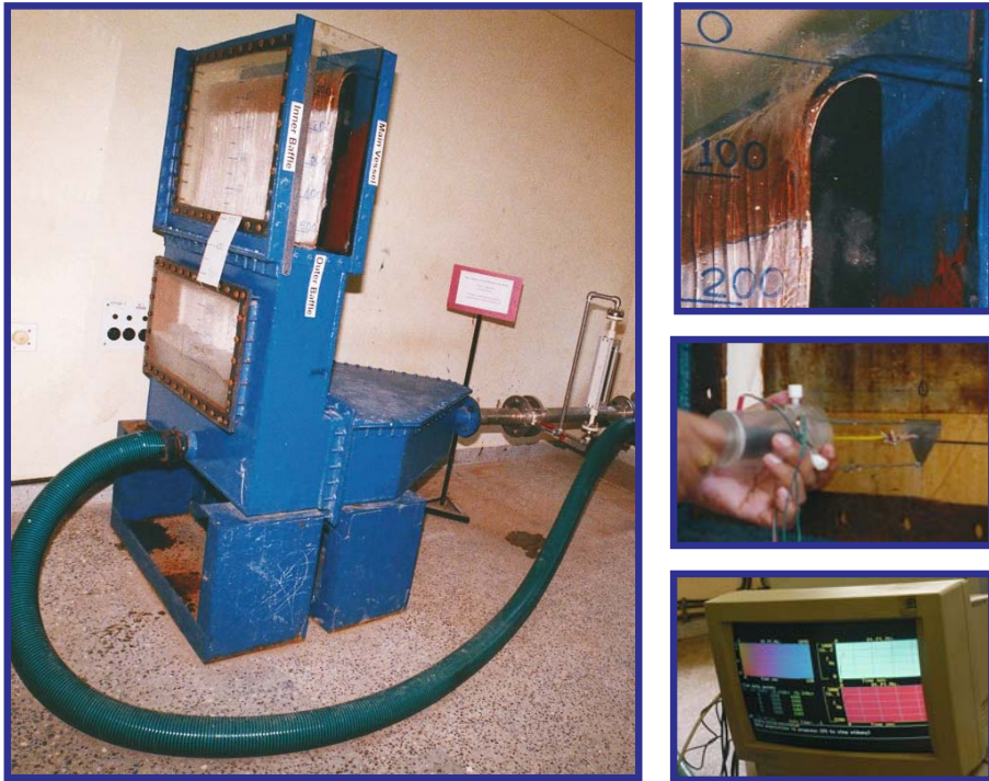
Figure 20. Weir-Crest testing full scale water model (left) and water film thickness being measured (right) by a special conductance probe connected to data acquisition system.
