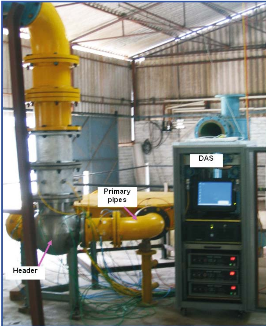
Figure 13. Experimental set-up to measure pressure loss in spherical header.
