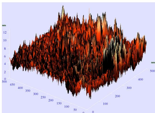
Fig. 8. AFM micrograph of the coating deposited by RF discharge.
