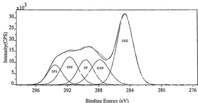
Fig. 6. XPS spectrum of the Teflon-like coating deposited with RF discharge.
