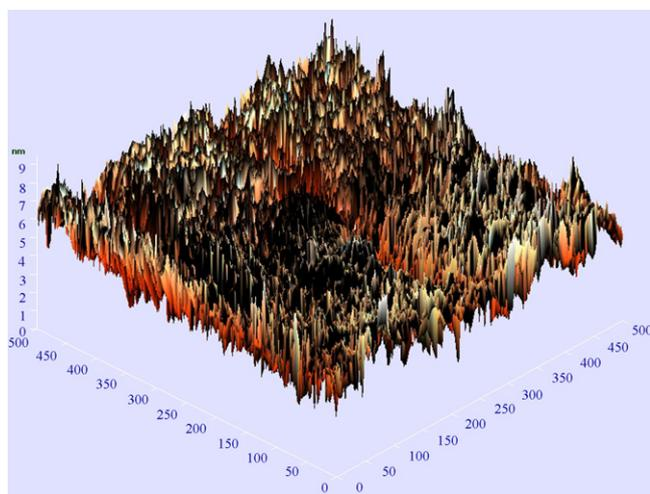
Fig. 7. AFM micrograph of the coating deposited by pulsed dc discharge.
