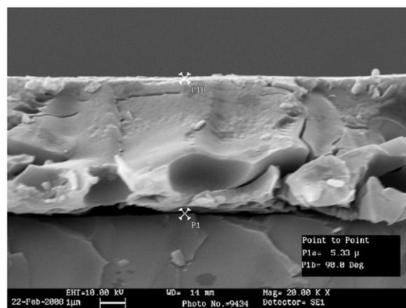
Fig. 4. SEM picture of Teflon-like coating deposited by RF PECVD.
