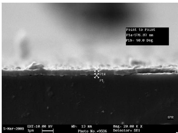
Fig. 3. SEM pictures of Teflon-like coating deposited by pulsed dc PECVD.
