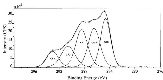
Fig. 5. XPS spectrum of the Teflon-like coating deposited with pulsed dc discharge.
