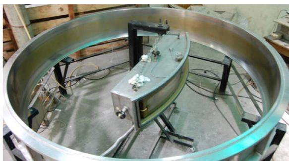
Fig. 2. Photograph of the SS shell deposited with Teflon-like coating, and the box coater.
