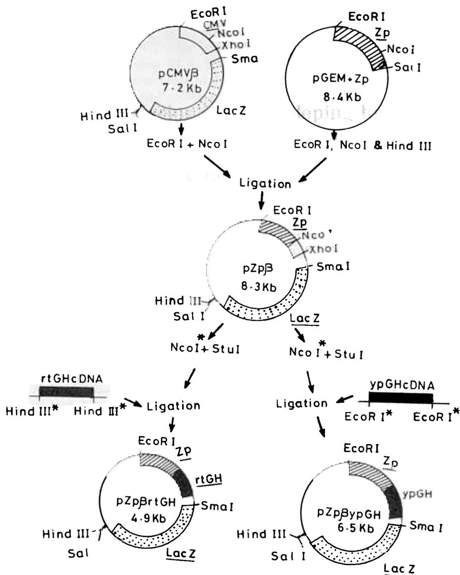
Figure 1. Protocol for construction of  $Zp\beta ypGH$  and  $Zp\beta rtGH$ . \*Fill-in reaction.
