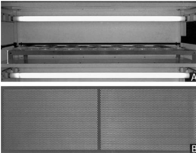
Fig. 2 A A shelf of a culture trolley showing the arrangements of culture plates. The white bar represents the height of the perforated stand (length=115 cm, width=40 cm, height=8 cm). The arrangement shown avoids the condensation of water on the lids of the petri dishes containing the cultures as direct heating of the bottom surface of the petri dishes from the lights placed on the lower shelf is eliminated. B Surface view of the perforated stand that is used to avoid condensation of water on the petri dish lids
