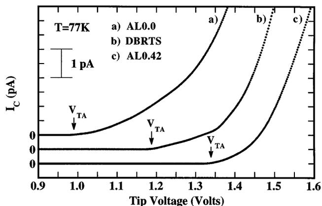
FIG. 2. BEEM  $I_C$ - $V$  spectra at 77 K for (a) AL0.0, (b) DBRTS, and (c) AL0.42.
