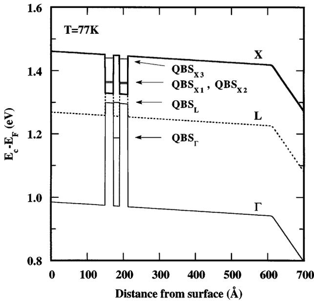
FIG. 3. DBRTS band profiles and QBS's for the  $\Gamma$ ,  $L$ , and  $X$  bands at 77 K.
