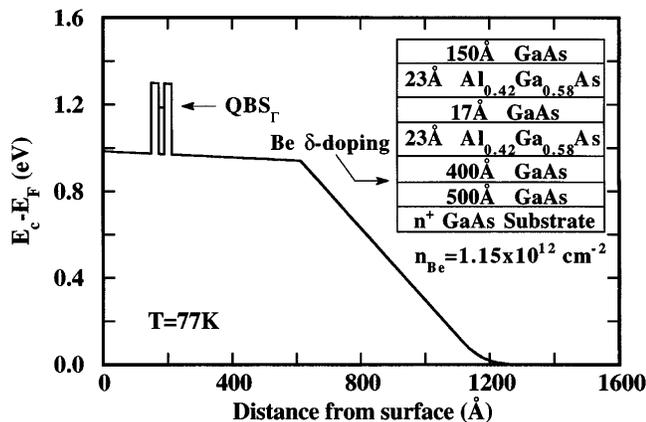
FIG. 1. DBRTS band profile at 77 K. The inset shows the sample structure.
