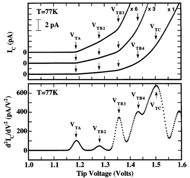
FIG. 4.  $I_C$ - $V$  and  $d^2I_C/dV^2$ - $V$  for the DBRTS at 77 K. The  $I_C$ - $V$  is magnified to clearly show the presence of additional structures beyond  $V_{TA}$ . The peaks in the  $d^2I_C/dV^2$ - $V$  correspond to the  $V_T$ 's in the  $I_C$ - $V$ .
