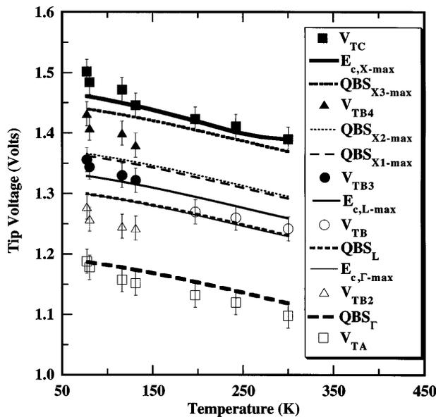
FIG. 6.  $T$  dependence of the calculated energetically favorable levels (see Fig. 3) and the observed  $V_T$ 's deduced from the peaks of the  $d^2I_C/dV^2-V$  in Fig. 5. Solid lines correspond to the band edges, whereas dashed (dotted) lines correspond to the QBS's.
