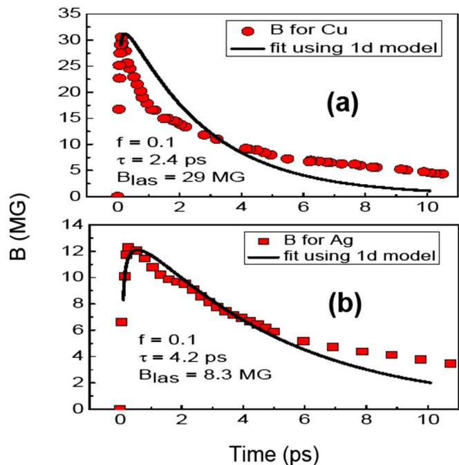
FIG. 4. (Color online) Magnetic field pulse profile for (a) Cu and (b) Ag,  $p$  polarized pump pulse.
