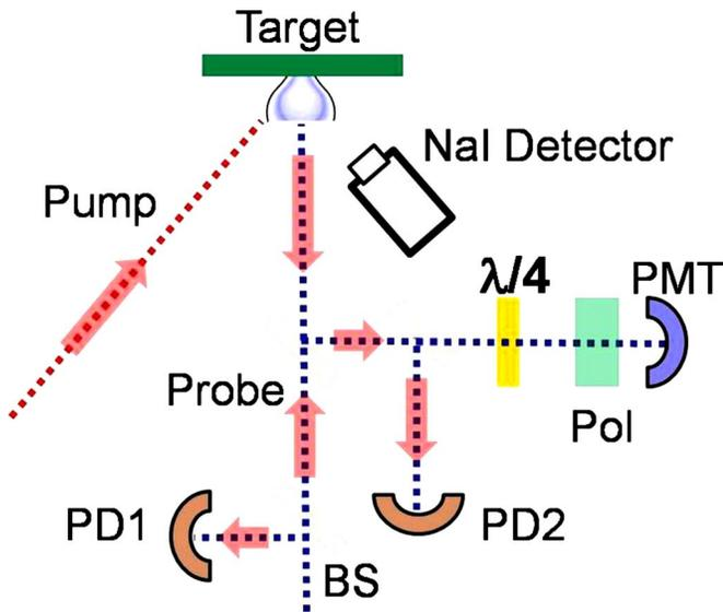
FIG. 1. (Color online) Experimental setup: beam splitter (BS), photodiodes (PD1, PD2), photomultiplier tube (PMT), quarter wave plate ( $\lambda/4$ ), and polarizer (Pol).
