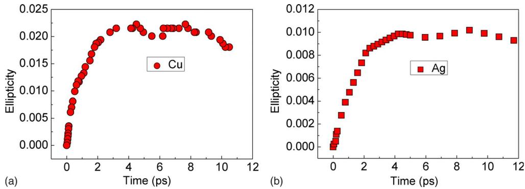
FIG. 3. (Color online) Induced ellipticity of probe as a function of delay time for Cu and Ag.
