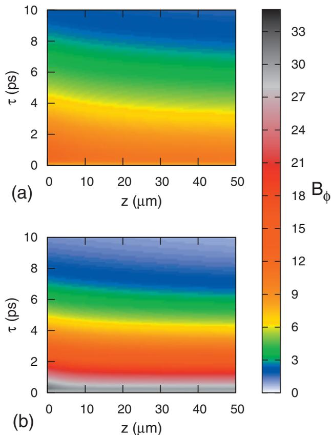
FIG. 5. (Color) The delay time ( $\tau$ ) and space ( $z$ ) dependence of the magnetic field  $B_\phi(z, \tau)$  in case of (a) Ag and (b) Cu using 1D model.
