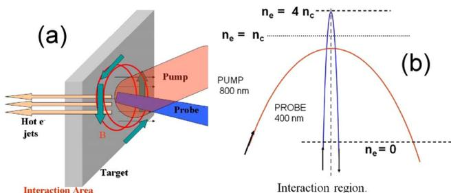
FIG. 2. (Color online) (a) Expanded view of interaction region. (b) The second harmonic probe pulse penetrates the region overdense for the pump pulse.
