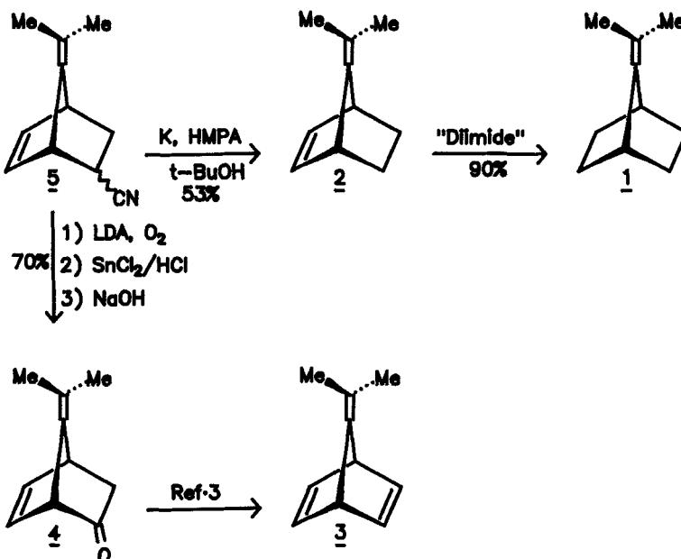
decyanation with K in HMPA following a procedure described by Normant's group<sup>6</sup> to furnish 2 (55%) in one step (cf. 4-5 steps used earlier).<sup>1a,3</sup> Diimide reduction on 2 proceeded smoothly and regioselectivity with reduction of the norbornene double bond to furnish 1 (90%).
