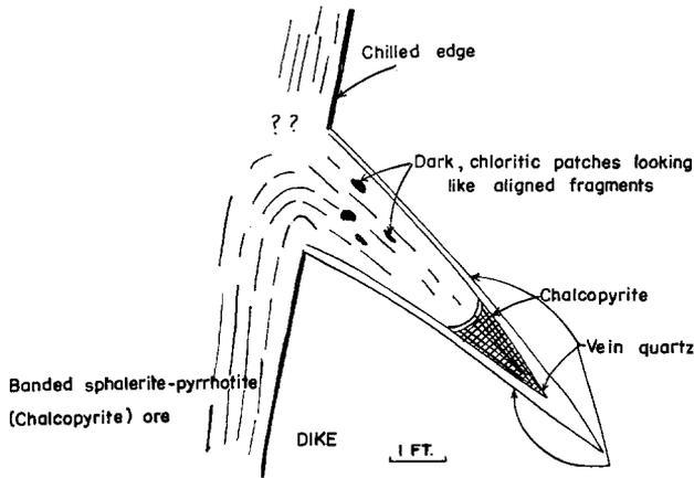
Fig. 15. Flowage of banded sulphide ore into a gash opening in a dyke. The opening, originally filled with quartz, was re-opened to accommodate plastically mobilized sulphide ore. Note (a) *continuity* of orebody sulphide bands into the opening, (b) chilled edge of the dyke, and (c) concentration of chalcopyrite at the tip of the opening. Deformation and regional metamorphism later than the post-ore dyke. 700 level, Joutel mine, Quebec, wall section
