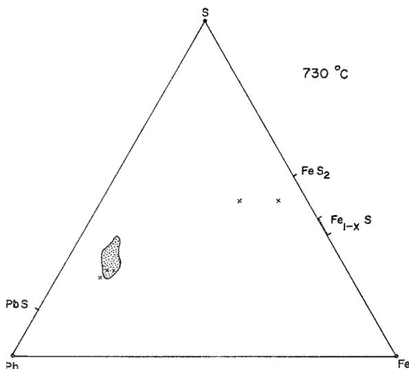
Fig. 1. 730 °C isothermal section of the system Fe-Pb-S, showing the ternary liquid field (Brett and Kullerud 1964) and the compositions of rheomorphic ore veins from Zawar mines, Rajasthan (indicated by cross marks)
