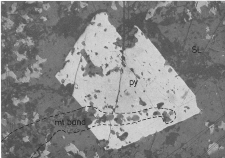
Fig. 11. Pyrite porphyroblasts (py) formed due to regional metamorphism. Note that the trail of magnetite inclusions within the porphyroblasts is *continuous* with the external S-plane defined by a magnetite band. Incident light, 150x Mattagami mine
