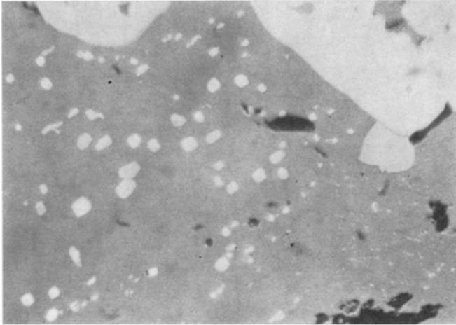
Fig. 8. Chalcopyrite exsolution 'cubes' in sphalerite, suggesting coalescence and high temperature modification due to heat. Ore from dyke contact, Normetal mine. Reflected light, 250x
