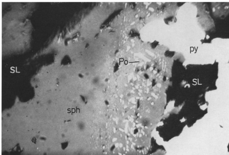
Fig. 3. Pyrrhotite 'ex-solution' blebs in sphalerite confined to pyrite-sphalerite contact, indicating reequilibration between the two minerals during subsequent heating by the dyke. Note decrease in size of blebs away from the boundary. Specimen two inches from contact, 4th level, Zawar mine. Reflected light, 300x. Py = pyrite, Po = pyrrhotite, Sph = sphalerite
