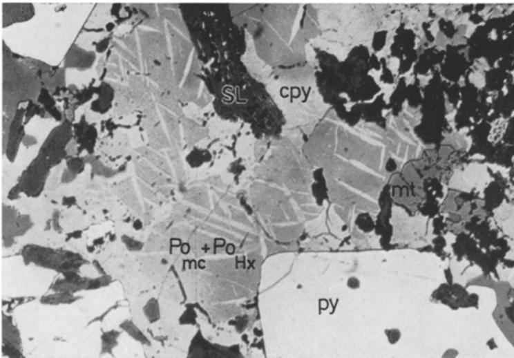
Fig. 13b. Micro-texture of 'normal' Geco ore. Pyrite (white), chalcopyrite (greyish white), twophase pyrrhotite (gray, with white lamellae), and some sphalerite and silicates. Location of sample shown in Fig. 13. Incident light, 50x
