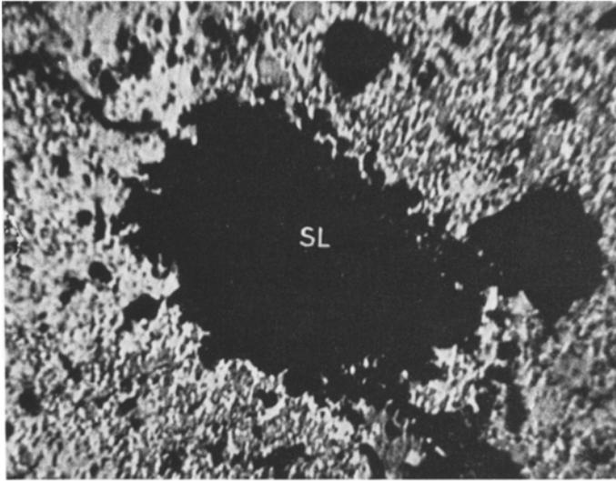
Fig. 13a. Micro-texture of the sulphide veins into the dyke, as shown in Fig. 13. Graphic (pseudoeutectoid?) intergrowth of sphalerite, chalcopyrite and pyrrhotite surrounding a corroded inclusion (black) of dyke material. Incident light 100x
