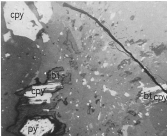
Fig. 18. Pseudomorphic replacement of biotite (bt) in a metamorphosed basic dyke by chalcocyanite (cpy), suggesting late mobilization of sulphides. Dyke post-ore, pre-metamorphic. Geco mine. Incident light, 250x
