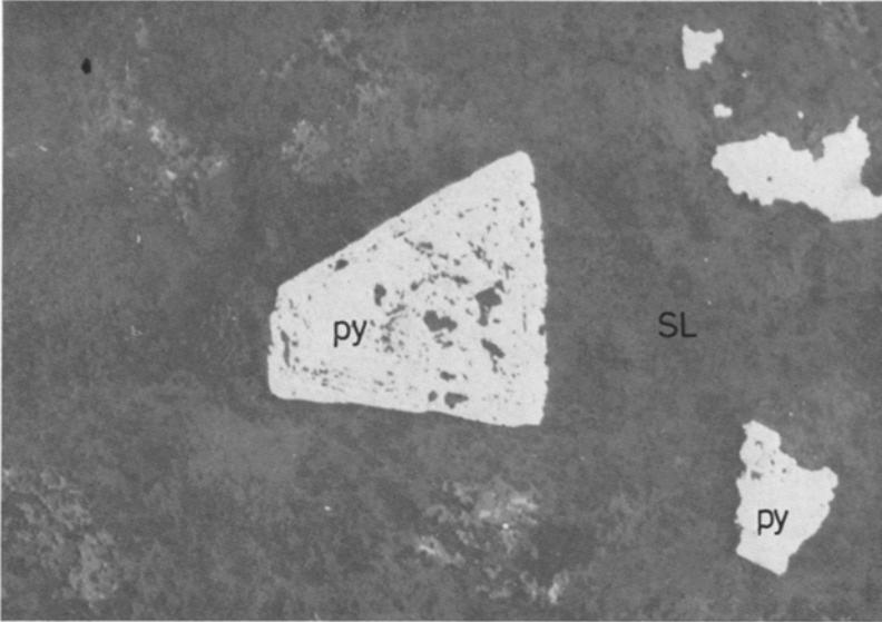
Fig. 10. Pyrite porphyroblasts (py) formed due to thermal metamorphism. The inclusions are zonally arranged, in contrast with those in Fig. 11. Incident light, 100x, Mattagami mine
