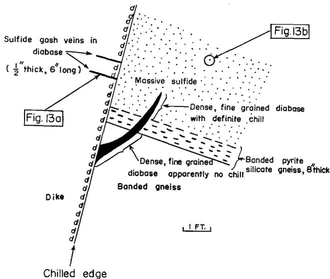
Fig. 13. Vertical section along 10-40 stope wall, Geco mine, Manitouwadge. Dyke apophyse cutting across concordant layers of biotite-gneiss and massive sulphide ores
