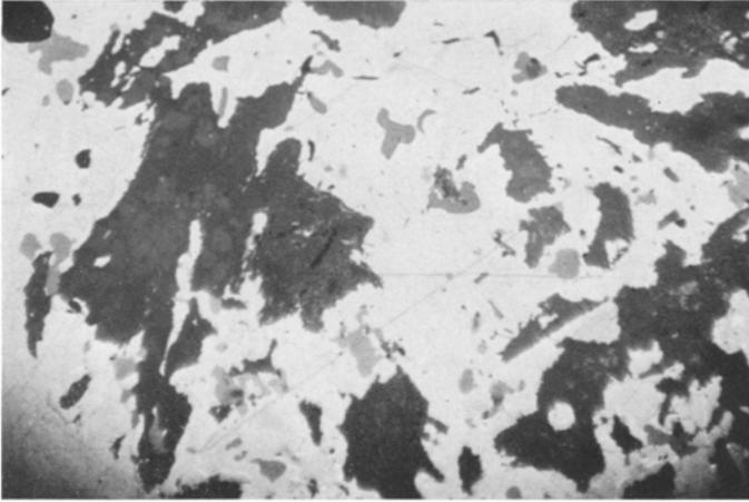
Fig. 7. Pyrrhotite coronas (white) around silicate islands (dark) floating in sulphide (sphalerite = light gray, chalcopyrite = white) matrix. Massive sulphide ore from dyke contact. Normetal mine. 80x, incident light
