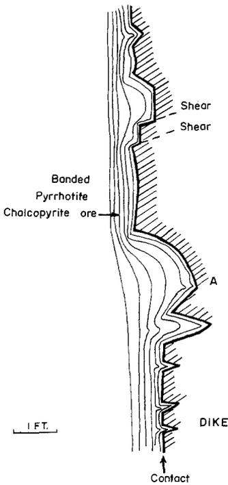
Fig. 16. Irregular dyke-ore interface caused by 'buckled' sulphide bands into fractures in the dike. Sulphide bands retain their continuity and gradually flatten out. Original gash-like nature of the curvature at "A" is betrayed by minute kinks at the tip of adjacent sulphide band. Note that the number of kinked bands is directly related to the size of the opening. Wall section, 1100 Level, Joutel mine, Quebec.
