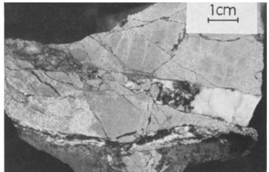
Fig. 6. Trails of pyroxene phenocrysts (dark spots, bottom), “frozen” in glassy matrix around a caught-up fragment (bottom, centre) of sulfide ore. Polished dyke-ore contact specimen. 300 L, Que-
