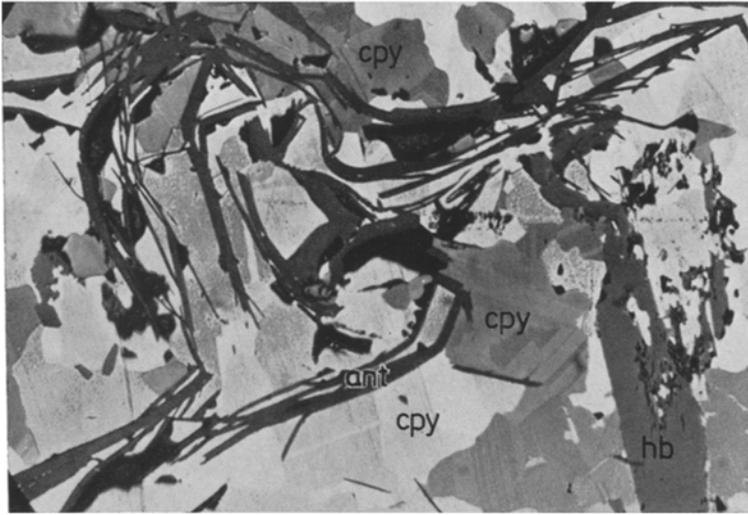
Fig. 12. Syntectonic crystallization of amphiboles (hb = hornblende, ant = anthrophyllite) in sulphide matrix. Chalcopyrite (gray and white) within fold arches and those 'replacing' thick hornblende prisms (centre, right) are recrystallized, untwinned. Willroy mine. Incident light, 80x, etched with aq. reg. vapour
