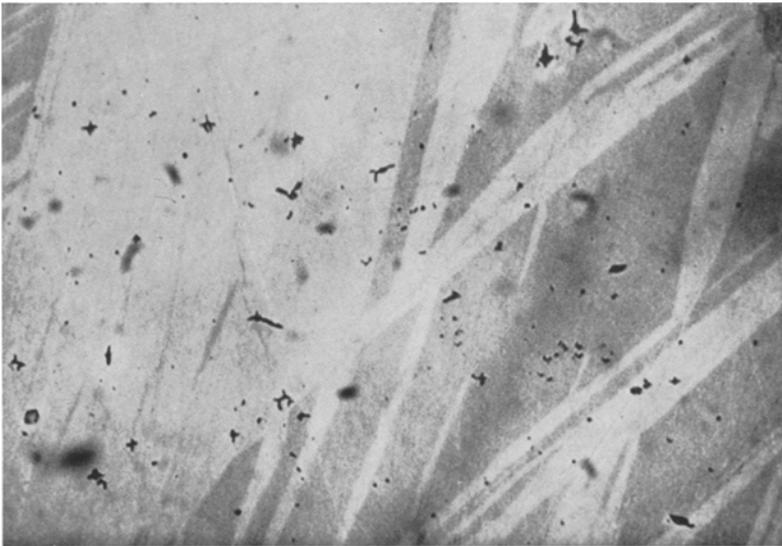
Fig. 9. Bi-convex twin lamellae and exsolved sphalerite starlets in chalcopyrite from ore "veins" in the dyke, Normetal mine. Both twinning and ex-solution are believed to have been promoted by deformation. Incident light, 450x, nicols partly crossed
