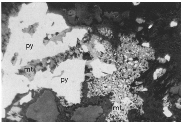
Fig. 4. Breakdown of pyrite(py) to magnetite(mt) along the contact of the ore body with the dyke. Horne mine, Noranda. Reflected light, 150x
