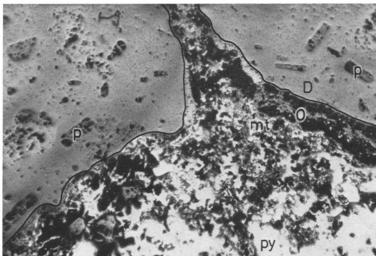
Fig. 17a. Photomicrograph of a dyke-ore contact specimen, unaffected by any later metamorphism. Pyrite dissociated to magnetite and ore vein injected into the dyke. Chilled margin with few plagioclase phenocrysts in glassy matrix. Horne mine, Noranda. Incident light, 200 x
