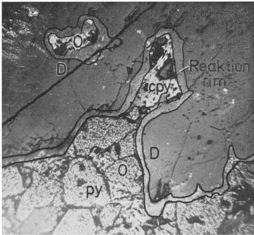
Fig. 17b. Photomicrograph of a dyke-ore contact specimen, affected by later metamorphism; dyke is recrystallized, chill obliterated, and a fine-grained reaction rim occurs along sulphide-silicate contact. Geco mine. Incident light, 100x
