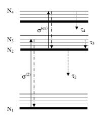
Fig. 4. A schematic energy level diagram for the Au clusters in the semi-molecular approximation. Downward transitions drawn close to the absorption transitions represent stimulated emission. Other decays are represented by their respective lifetimes,  $\tau_n$ .
