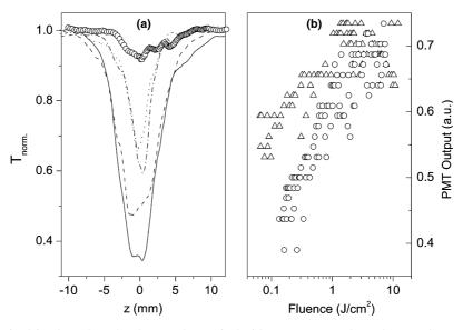
Fig. 2. (a) z-scan curves obtained for the 29 kDa Au clusters when excited with 532 nm, 7 ns pulses. The mean laser energy reaching the sample is  $38 \mu$ J. Linear transmissions are: solid curve, 0.20; dash, 0.3; dash-dot, 0.47 and dot, 0.67. Circles represent pure toluene. (b) Induced scattering signals obtained from the PMT, as a function of the input laser fluence. Linear transmissions are: circles, 0.20; triangles, 0.67.
