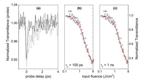
Fig. 5. (a) Transmission recovery of the Au<sub>140</sub> clusters when excited and probed with 400 nm, 100 fs pulses. Solid curve, pure toluene; dashed curve, hexanethiol protected cluster; dotted curve, dodecanethiol protected cluster. (b,c) Normalized transmittance of the Au@hexanethiol clusters with input laser fluence. Sample linear transmission is 0.2. Solid curves are numerical fits obtained for two different values of  $\tau_2$ .
