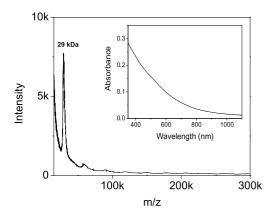
Fig. 1. MALDI-TOF spectrum of column separated Au@hexanethiol cluster compound with the matrix, indole acrylic acid (ratio 1:5) showing the presence of 29 kDa clusters exclusively. A minor peak due to the dimer formed during the ionization process [11] is also seen. *Inset*: Optical absorbance spectrum of the same sample, showing an extremely weak surface plasmon resonance around 523 nm.
