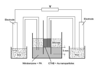
Fig. 1. Schematic of the experimental setup used for studying potential oscillations. 5 mm of the 2 cm diameter tube is dipped into the organic solution and the dipped end of the tube is given a notch of 1 mm. The cell is completed using two salt bridges and  $Ag/Ag^+$  electrodes. The monolayer is formed at the CTAB-nitrobenzene interface.
