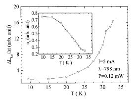
FIG. 2. Temperature dependence of  $\Delta L_{\rm kin}/\Delta t$  for  ${\rm La_{1.85}Sr_{0.15}CuO_4}$  thin film. The inset shows the square root of  $1/\Delta L_{\rm kin}/\Delta t$ , which is proportional to n if we assume  $\Delta n_s/\Delta t$  is temperature independent or weakly temperature dependent.
