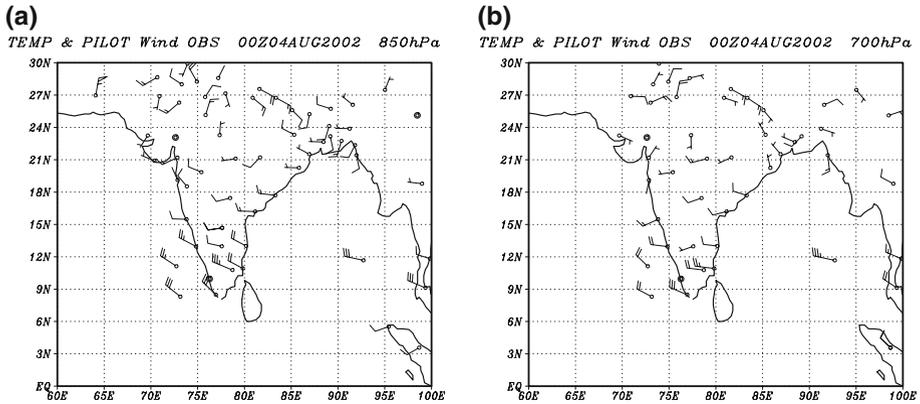
**Fig. 2** RS/RW and pilot balloon wind observations at 0000 UTC on 4th August 2002 (a) 850 hPa (b) 700 hPa
