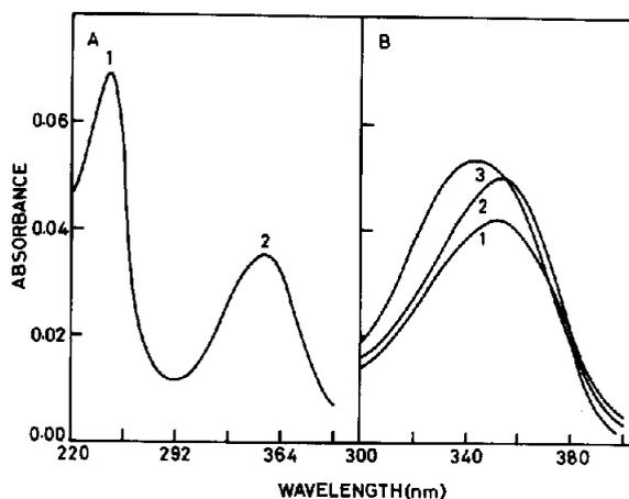
Fig.2. (A) Ultraviolet absorption spectra of colchicine ( $2.27 \times 10^{-6}$  M) in water. Absorption maxima:  $\lambda_{\max 1} = 247$  nm;  $\lambda_{\max 2} = 353$  nm. (B) Absorption spectra of colchicine ( $2.7 \times 10^{-6}$  M), desacetamidocolchicine ( $2.8 \times 10^{-6}$  M) and AC compound ( $3 \times 10^{-6}$  M) in assembly buffer. (1) Colchicine,  $\lambda_{\max} = 353$  nm; (2) desacetamidocolchicine,  $\lambda_{\max} = 353$  nm; (3) AC compound,  $\lambda_{\max} = 341$  nm.
