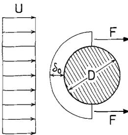
Fig. 1. Schematic representation of the elastic boundary layer in front of a bluff body
