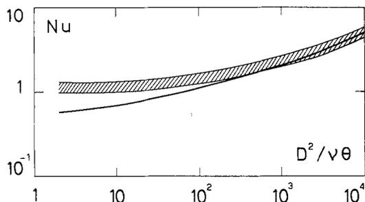
Fig. 3. Heat transfer correlation. The shaded area represents the data by *James and Acosta*
