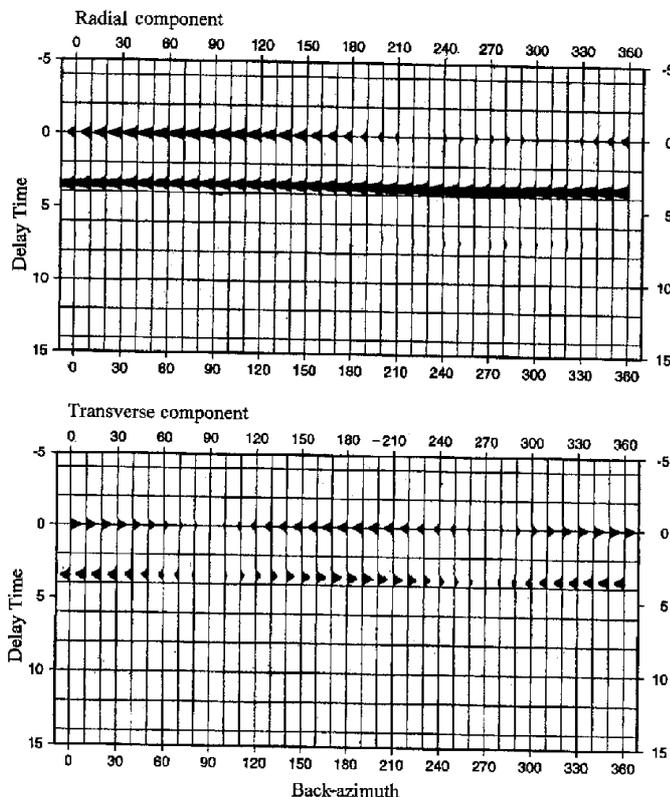
**Figure 3.** 2D synthetic radial and transverse RFs showing the effects of dipping interfaces and their diagnostics, as described in the text. The computations are made for a Moho with a strike of 180° and dip of 15°. Note the swerve in *Ps* phase close to 5 s in the radial RF showing clear azimuthal dependence, and change in amplitude and polarity of the *Ps* phase in transverse RF and its periodicity.
