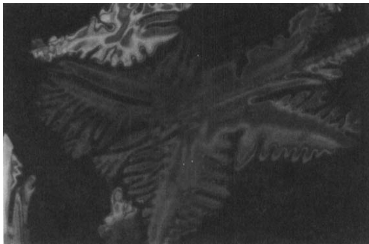
FIGURE 4 Dendritic growth of the B_1 phase in a mixture with 50 mol % of BC12 at 117.1^\circ\text{C} , crossed polarizers, ( \times 300 )
