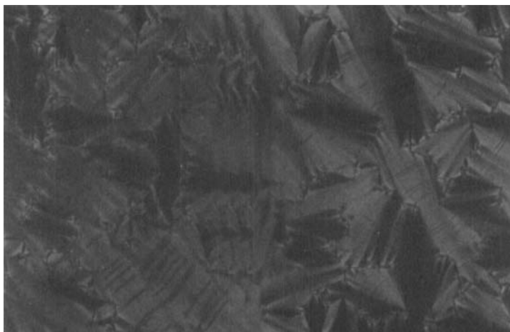
FIGURE 6 Focal conic texture of the B_6 phase in a mixture with 25 mol % of BC12 at 115°C, crossed polarizers, ( \times 240 ) See Color Plate XLIII at the back of this issue.
