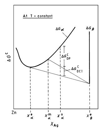
*Figure 9* Schematic diagram illustrating the principle of determination of the available chemical driving force for DP ( $\Delta G_{DP}^c$ ) and DCI ( $\Delta G_{DCI}^c$ ) from the chemical free-energy change ( $\Delta G^c$ ) versus composition ( $x_{Ag}$ ) diagram for the Zn–Ag system.
