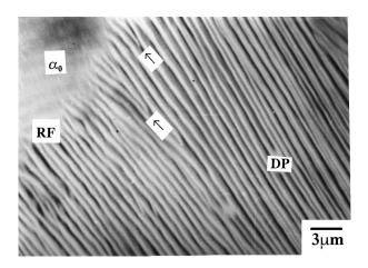
*Figure 1* A typical DP colony formed at 433 K after 2 h. The arrowheads illustrate a possible mechanism of maintaining constancy of  $\lambda_{DP}$  (at a given *T*) by branching of the  $\beta$ -lamellae.
