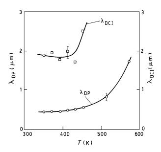
*Figure 6* Variation of interlamellar spacing in DP ( $\lambda_{DP}$ ) and DCI ( $\lambda_{DCI}$ ) versus isothermal ageing temperature (*T*).
