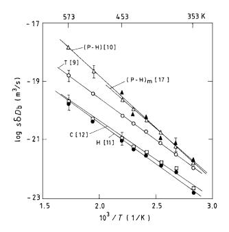
*Figure 11* Arrhenius plot of grain-boundary chemical-diffusivity triple product  $(s\delta D_b)$  derived from various analytical models. Key: Turnbull [9], (T); Petermann–Hornbogen [10], (P–H); Hillert [11], (H); Cahn [12], (C); Petermann–Hornbogen, modified by Fournelle [17], (P–H)<sub>m</sub>.
