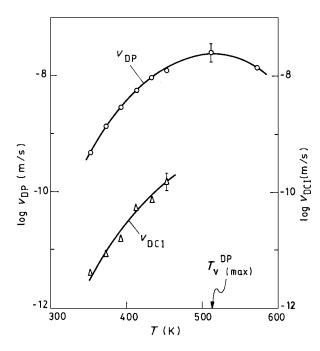
*Figure 5* Variation of the RF migration velocity during DP ( $v_{DP}$ ) and DCI ( $v_{DCI}$ ) as a function of isothermal ageing temperature (*T*).  $T_{v(max)}^{DP} = 513$  K corresponds to  $v_{max}$  (see text).
