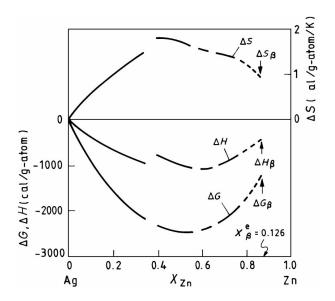
*Figure 8* Determination of the free energy of formation of the  $\beta$  phase  $(\Delta G_{\beta})$  at the required composition of  $x_{\beta}^{e} = 0.126$  by suitable extrapolation of the changes in enthalpy  $(\Delta H_{\beta})$  and entropy  $(\Delta S_{\beta})$  data reported by Hultgren *et al.* [35] for T = 873 K.
