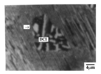
*Figure 4* Initiation of an isolated DCI colony at the intersection between a former DP colony with the free (external) surface (indicated by an arrow-head).
