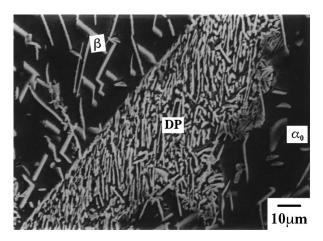
*Figure 2* Formation of Widmannstätten  $\beta$  in the  $\alpha_0$ -matrix by continuous/matrix precipitation as a parallel mode of decomposition of  $\alpha_0$  along with DP at T = 433 K, t = 4 h.
