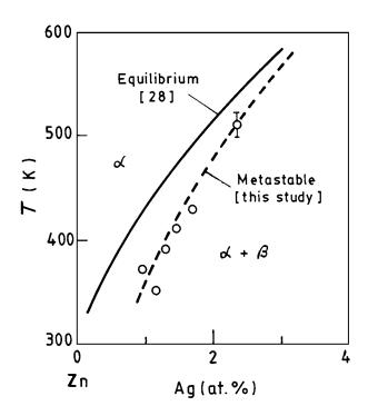
*Figure 7* Metastable solvus curve for the Zn–Ag system indicating the average solute concentration  $(x_{\alpha}^{m})$  in the Zn–rich  $\alpha$  phase following DP at a given *T*. The equilibrium solvus line [28] is shown here for comparison.
