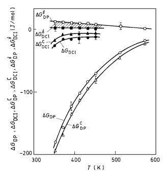
Figure 10 Variation of the overall driving force for DP and DCI along with their constituent components in terms of the respective Gibbs freeenergy changes as a function of the isothermal ageing temperature (T).
