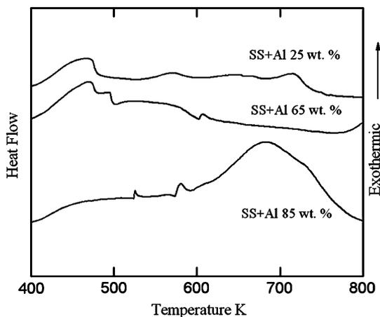
Fig. 12—DSC patterns of 316SS with 25, 65, and 85 wt pct Al alloy powder after ball milling of 50 h.
