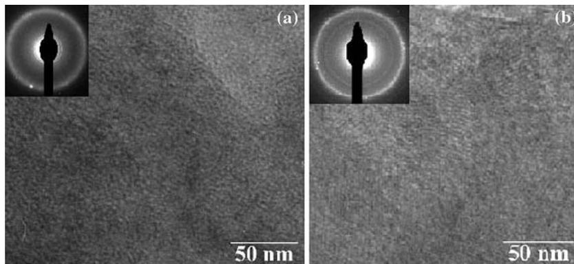
Fig. 6—(a) HRTEM images of 316SS and 65 wt pct Al powder blend showing predominantly amorphous microstructures following 30 h of ball milling and the corresponding SADP (inset). (b) HRTEM images of 316SS and 65 wt pct Al powder blend showing nanocrystalline grains following 50 h of ball milling. The SAD (inset) confirms the matrix as a nanocrystalline fcc phase.
