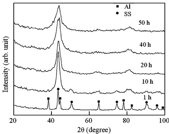
Fig. 3—XRD patterns of a powder mixture of 316SS and 25 wt pct Al subjected to planetary ball milling for different cumulative milling times.
