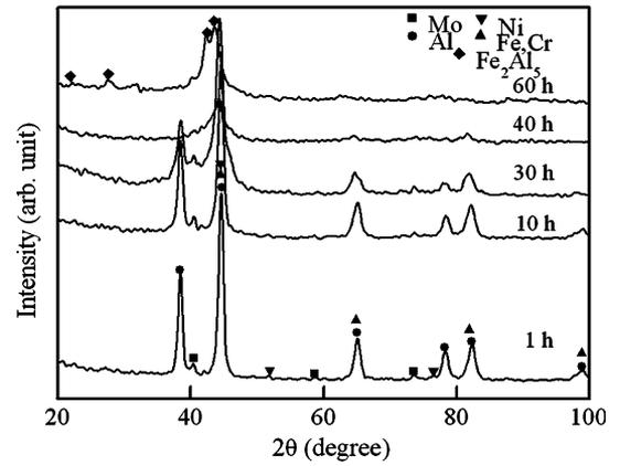
Fig. 7—XRD patterns of a powder mixture of elements with equivalent 316SS composition and 65 wt pct Al subjected to planetary ball milling for different cumulative milling time.
