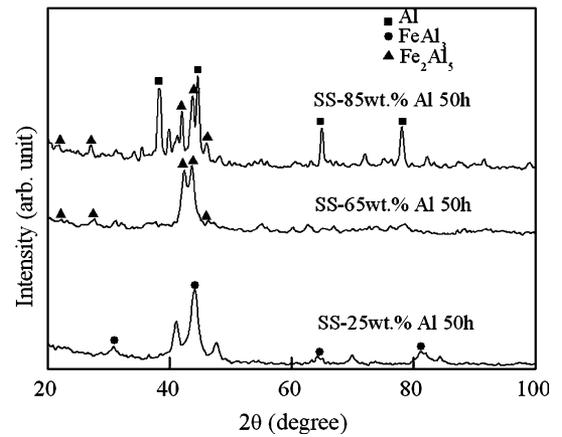
Fig. 13—XRD patterns of the ball-milled samples after isothermal treatment at 775 K for 2 h.
