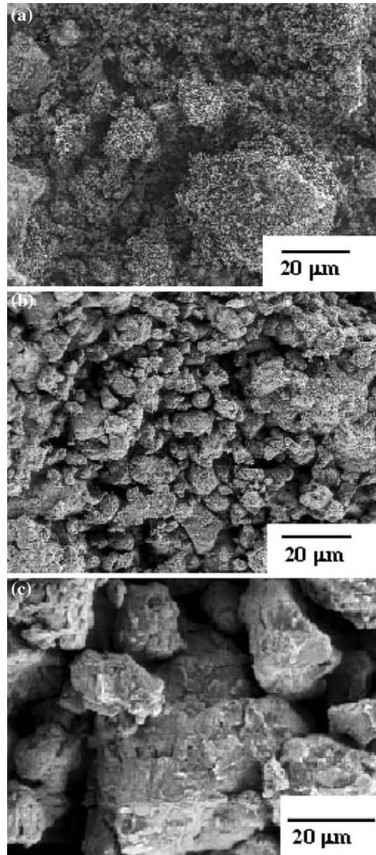
Fig. 15—Scanning electron micrograph of green-compacted samples of powder blends consisting of (a) 316SS + 85 wt pct Al, (b) 316SS + 65 wt pct Al, and (c) 316SS + 25 wt pct Al.
