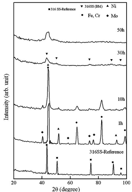
Fig. 1—XRD pattern obtained after ball milling of elemental blend having nominal composition comparable to 316SS. The XRD pattern of the 316SS alloy is appended as a reference for indexing the fcc ball-milled product after 30 h.
