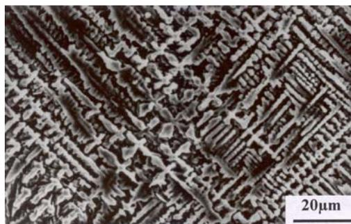
Figure 2: Scanning electron micrograph (SEI) of the top surface of laser nitrided Ti-6Al-4V lased with a power of 700 W.
