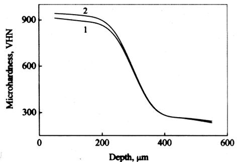
Figure 5: Variation of microhardness with depth from the surface of laser surface nitrided Ti-6Al-4V with a power of 800W (plot 1) and 600W (plot 2) respectively
