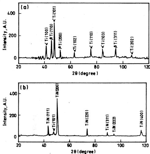
Figure 4: X-ray diffraction profile of (a) as received, (b) laser surface nitrided (with a power 600W) Ti-6Al-4V.
