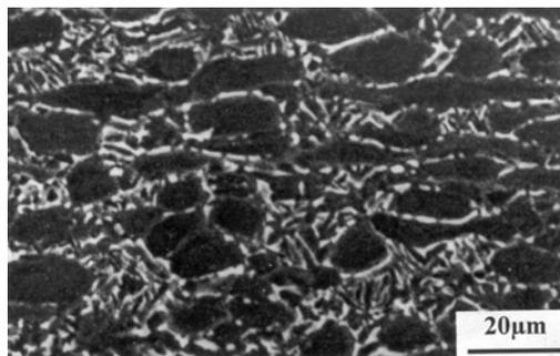
Figure 1: Scanning electron micrograph (SEI) of as received Ti-6Al-4V
