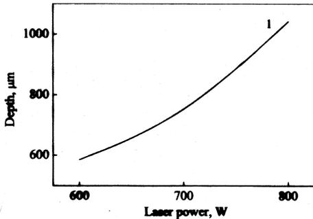
Figure 3: Variation of depth of nitriding with applied laser power.
