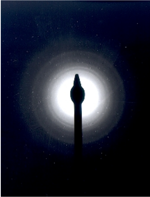
Fig. 4. Amorphous halo in the TEM dark filed image of the \text{Al}_{65}\text{Cu}_{20}\text{Nb}_{15} alloy following mechanical alloying for 40 h.
