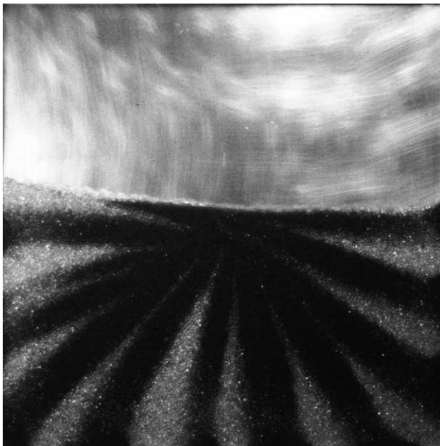
Fig. 3. Pattern formation resulting from a competition between size segregation and mixing in a rotating container in the continuous flow regime [29]. Reproduced with permission from Proc. Natl. Acad. Sci. U. S. A.
