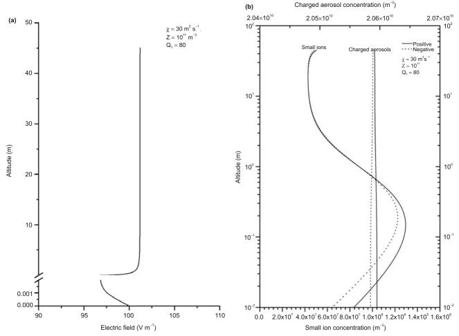
Figure 1. (a) Vertical profiles of electric field and (b) small ion concentration and charged aerosol concentration for  $Z = 10^{11} \,\mathrm{m}^{-3}$  and  $\chi = 30 \,\mathrm{m}^2 \,\mathrm{s}^{-1}$ .
