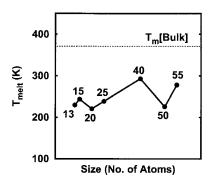
FIG. 8. The melting temperature as a function of size. The melting temperature in bulk  $(T_m[Bulk])$  is 370 K.
