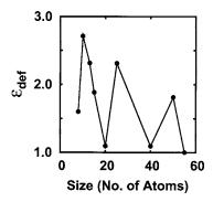
FIG. 3. The deformation parameter  $\varepsilon_{def}$  as a function of size for the ground-state geometries.  $\varepsilon_{def}$ =1 indicates a spherical system and  $\varepsilon_{def}$ >1 indicates a quadrupole deformation.
