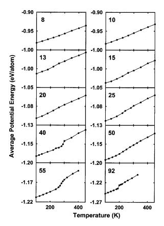
FIG. 6. The averaged potential energy (Caloric curve) as a function of temperature.
