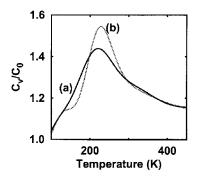
FIG. 1. The specific heat of the  $Na_{20}$  cluster with simulation time of (a) 150 ps and (b) 90 ps as a function of temperature.
