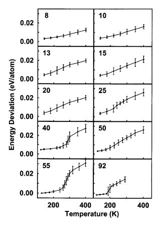
FIG. 9. The deviation of total energy from that of the harmonic limit as a function of temperature. The error bar is the standard error at each temperature.
