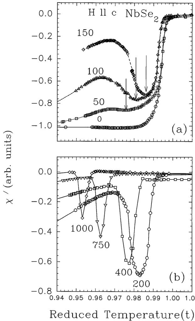
FIG. 1. Temperature variation of the in-phase ac [ $f = 21$  Hz,  $h_{ac} = 2$  Oe (rms)] susceptibility  $\chi'_H(T)$  for  $H||c$  in a single crystal of  $2H-NbSe_2$  [ $T_c(0) \approx 7.1$  K]. The arrows identify the positions ( $T_{\text{peak}}(H)$ ) of negative peak in  $\chi''(T)$  plots.
