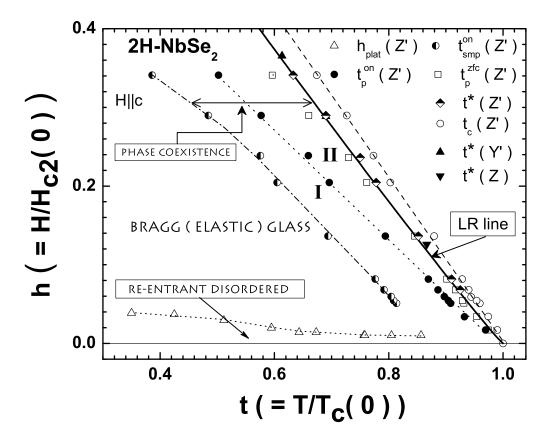
FIG. 5: A magnetic phase diagram in a typically weakly pinned single crystal Z' of 2H- $NbSe_2$  drawn in terms of reduced field (h) and temperature (t). The theoretical spinodal line based on the work of Li and Rosenstein [31] has also been drawn as a solid line. The rest of the lines passing through various data sets are to guide the eye. Following Ref. [11], we have also included the data related to the limiting (spinodal) temperature in the other 2H- $NbSe_2$  crystals (Y') and Z.
