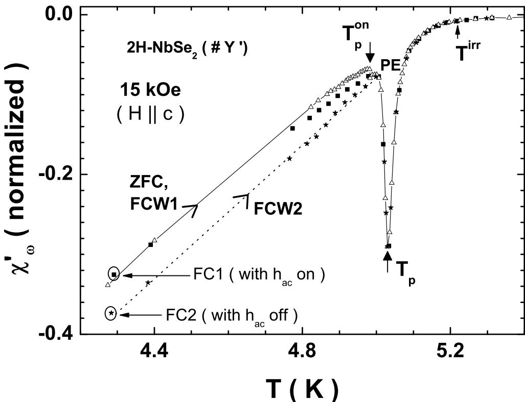
FIG. 1: In-phase ac susceptibility ( $\chi'_\omega$ ) data at  $H = 15$  kOe( $\parallel c$ ) and in  $h_{ac}$  of 0.5 Oe (rms) in the crystal  $Y'$  ( $T_c(0) \approx 7.25K$ ) of  $2H$ -NbSe<sub>2</sub> for different thermomagnetic histories, as indicated. While obtaining the FC1 and FC2 states, the  $h_{ac}$  remained *on* and *off*, respectively.
