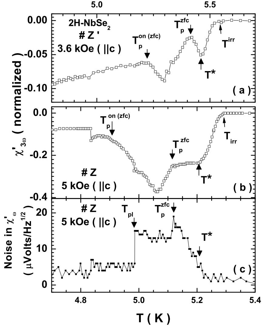
FIG. 4: The panels (a) and (b) show  $\chi'_{3\omega}(T)$  data at 3.6 kOe and 5 kOe for  $h_{ac} = 2.5$  Oe (rms) in the crystal  $Z'$  and  $Z$ , respectively. The panel (c) displays the noise in  $\chi'_{\omega}(T)$  recorded with a wide band filter at 5 kOe with  $h_{ac} = 0.5$  Oe(rms) and at a frequency of 211 Hz in the crystal  $Z$ . The positions of the respective  $T_p^{\text{on}}$  (&  $T_{\text{pl}}$  [16]) and  $T_p$  values (see text) have been marked in the different panels.
