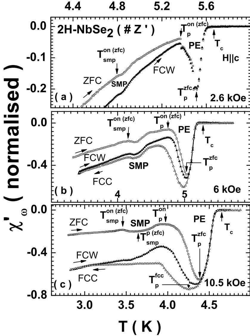
FIG. 2:  $\chi'_\omega(T)$  data ( $h_{ac} = 1.5$  Oe(rms)) for different thermomagnetic histories at the dc fields ( $H \parallel c$ ) indicated in the crystal  $Z'$  ( $T_c(0) \approx 6.0K$ ) of  $2H\text{-NbSe}_2$ . The anomalies corresponding to the SMP and the PE have been identified and the respective positions of  $T_{smp}^{on}$ ,  $T_p^{on}$ ,  $T_p^{zfc}$  and  $T_c$  have been marked.
