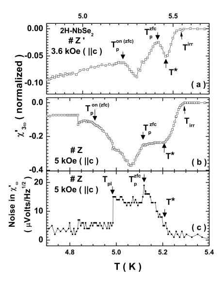
FIG. 4: The panels (a) and (b) show  $\chi'_{3\omega}(T)$  data at 3.6 kOe and 5 kOe for  $h_{ac}=2.5$  Oe (rms) in the crystal Z' and Z, respectively. The panel (c) displays the noise in  $\chi'_{\omega}(T)$  recorded with a wide band filter at 5 kOe with  $h_{ac}=0.5$  Oe(rms) and at a frequency of 211 Hz in the crystal Z. The positions of the respective  $T_p^{on}$  ( &  $T_{pl}$  [16]) and  $T_p$  values (see text) have been marked in the different panels.
