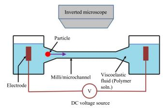
Figure 5. Schematic showing a possible experimental set-up to test the prediction of the theoretical analysis reported herein. The set-up consists of a fluidic conduit with two reservoirs at the two ends, wherein two electrodes have been placed to impose a DC electric field. Particle motion can be captured using an inverted microscope placed above the set-up. Polystyrene beads may be used as particles and Polyethylene solution can be used as a viscoelastic medium.
