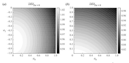
Figure 4. (a) Contour plot of  $\mathcal{U}/\mathcal{U}_N$  vs  $a_0$  and  $a_1$  (<0), for  $De=1, \lambda_1=1, \lambda_2=0.5, \beta=1, \bar{\zeta}_0=0.25$ . (b) Same contour plot, but for  $a_1>0$ .
