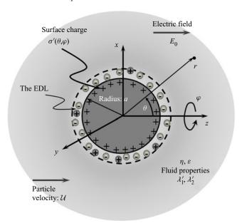
Figure 1. Schematic of a spherical particle of radius a, carrying an arbitrary surface charge density  $\sigma'(\theta, \varphi)$ . The particle is translating with velocity  $\mathcal{U}'\hat{e}_u$  in a viscoelastic medium, subject to an externally applied electric field (magnitude far from the particle  $E_0$ ) along the z direction. The fluid has viscosity  $\eta$ , relaxation time  $\lambda'_1$ , retardation time  $\lambda'_2$  and permittivity  $\varepsilon$ .
