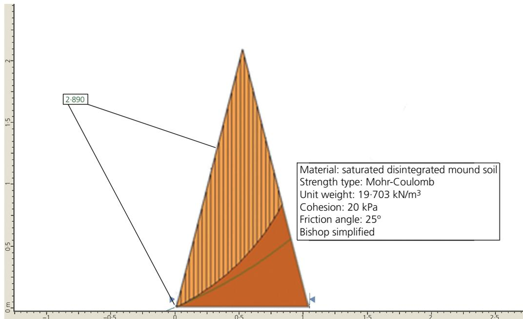
**Figure 10.** Slope stability analysis performed with the remoulded termite mound soil properties obtained from direct shear using Slide to obtain the factor of safety against failure
