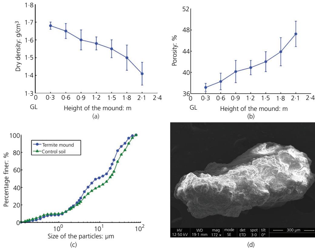
**Figure 2.** (a) Variation of dry density in mound with elevation. The abscissa shows the height of the termite mound from ground level (GL). (b) Variation of porosity at different levels of the mound. The abscissa shows the height of the termite mound from ground level (GL). (c) Cumulative particle size distributions of mound soil
