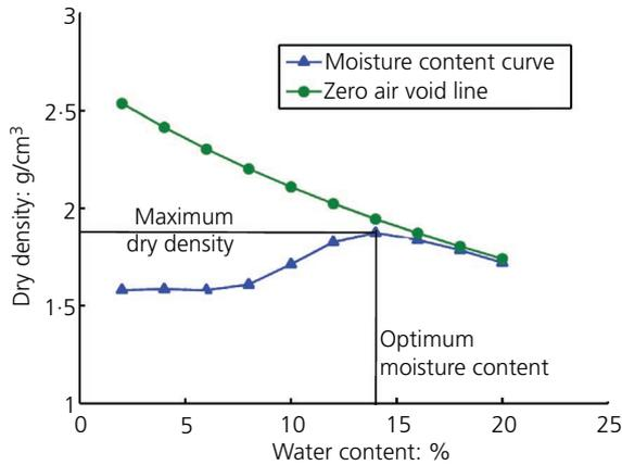
**Figure 5.** Compaction results indicating the maximum dry density and OMC of the reconstituted mound soil. The experiments were performed by applying a controlled energy to the soil-water mixture to achieve the densest packing possible
