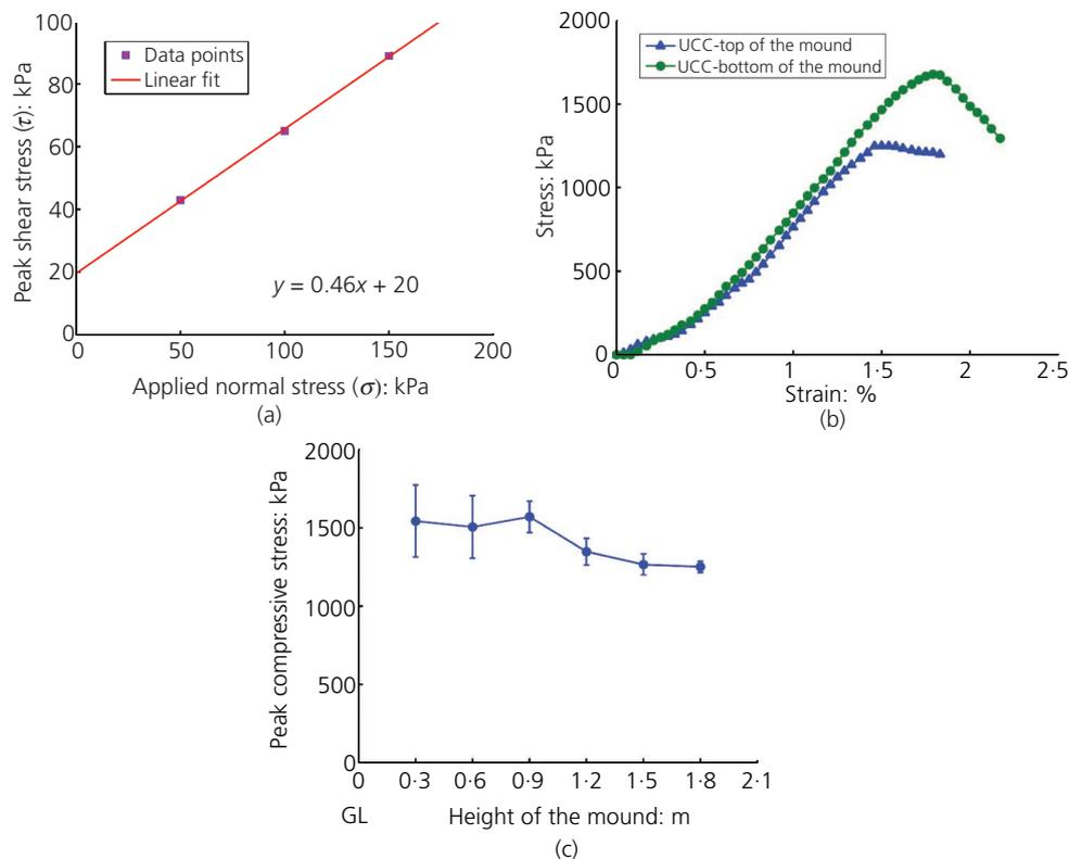
**Figure 7.** (a) Direct shear test performed at three normal loads to determine the shear strength parameters (cohesion and friction angle). The y intercept gives the cohesion value, and the slope of the linear fit gives the friction angle. (b) Variation of stress against strain obtained by testing under unconfined compression (UCC).
