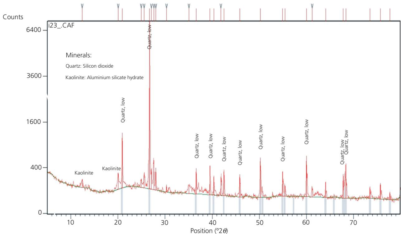
**Figure 6.** The inorganic mineralogical composition of the termite mound soil as illustrated with a sample XRD result
