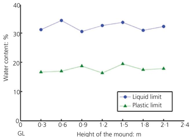
**Figure 4.** Atterberg's limits at obtained from different locations of the mound. The liquid limit and the plastic limit are almost constant throughout the mound
