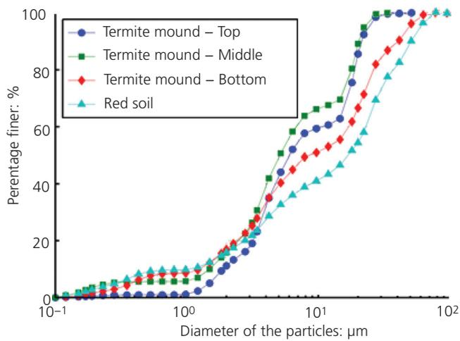
**Figure 3.** Particle size distributions of the mound soil (top, middle and bottom) and the control soil. The mean particle size of the termite mound soil is three to four times smaller than that of the control soil
