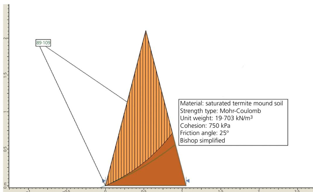
**Figure 9.** Slope stability analysis performed at on-site conditions using the limit equilibrium package Slide to obtain the factor of safety against failure. The value of 89.109 indicates the safety factor
