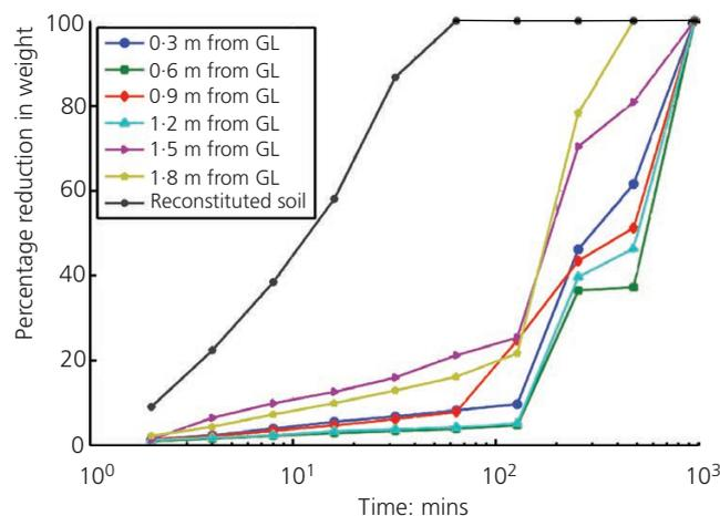
**Figure 8.** Weathering experiments (alternate wetting and drying) to determine the stability of the mound performed on the mound soil obtained from different parts of the mound with increasing time intervals (wetting time interval) and compared with the reconstituted soil. The legend in the figure indicates that the samples were collected at different heights from ground level (GL)
