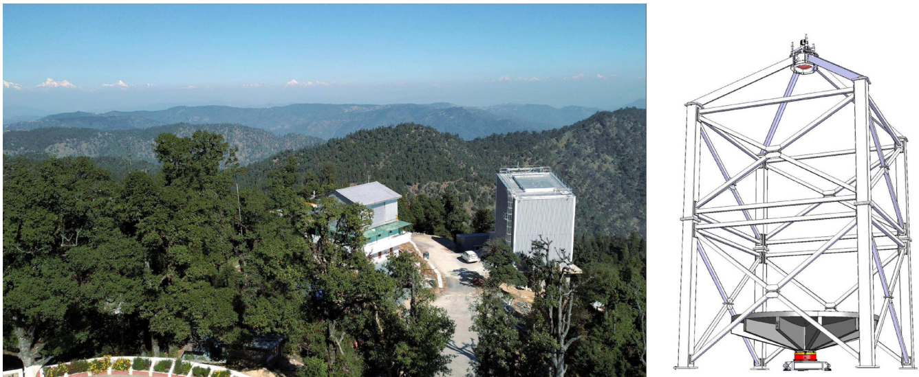
Figure 1. Left panel: Panoramic view of the ILMT site. The 1.3-m DFOT and the 4-m ILMT are in the middle and right sides, respectively, in this image. Right panel: Major components of the ILMT. Here, the container is grey, the air bearing is red, the three-point mount (white) sits below the air bearing, and the vertical steel frames (white) hold the corrector and the CCD camera at the top. The tentative size and other parameters of the telescope are listed in Table 1. Note the nice view on the Himalayan chain in the background of the left photograph.
