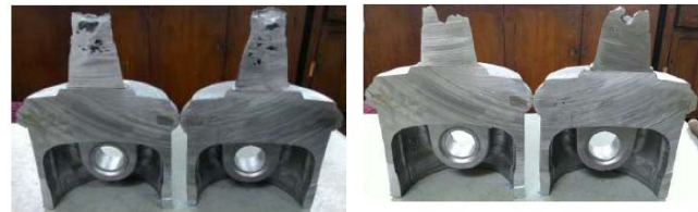
Figure 10. Piston casting cross section sample when pouring metal temperature is about 740°C and 720°C respectively.
