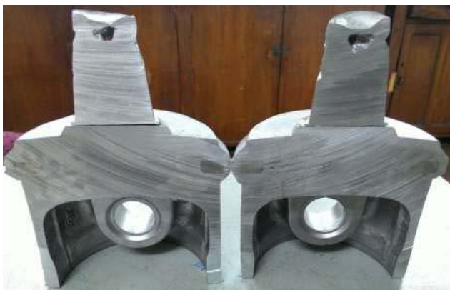
Figure 9. Piston casting Cross section with 4C riser sleeve size.
