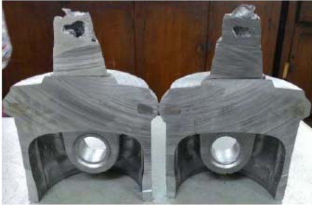
Figure 12. Piston casting cross section sample when solidification time 120 secs is given.
