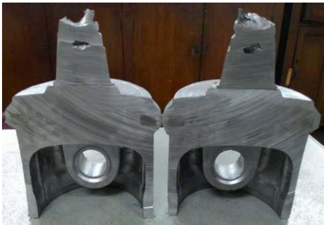
Figure 8. Piston casting Cross section with 4 riser sleeve size.
