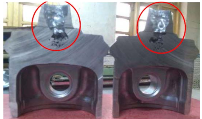
Figure 5. Cross section of second cavity piston casting at low centre core temperature with gross crown shrinkage.
