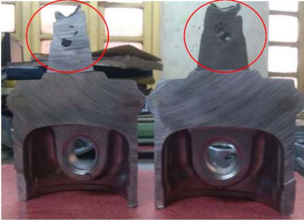
Figure 7. Cross section of 2nd cavity piston casting at high centre core temperature.
