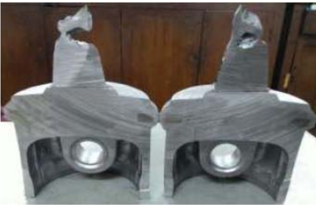
Figure 13. Piston casting cross section sample when solidification time 150 secs is given.
