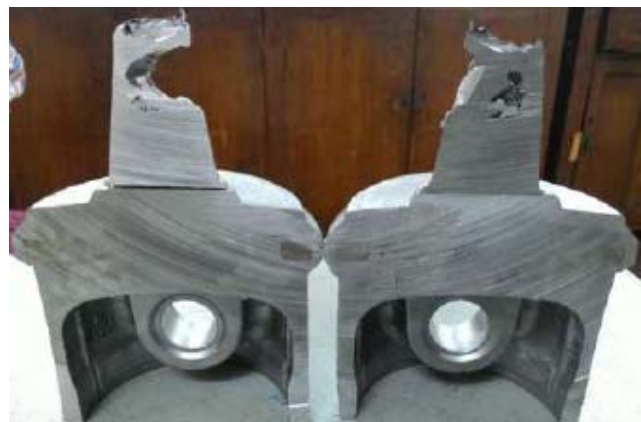
Figure 11. Piston casting cross section sample when solidification time 90 secs is given.
