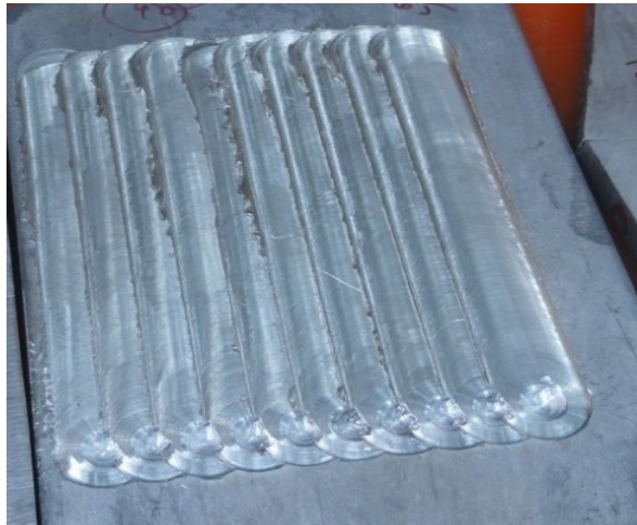
Fig. 1 Photograph of AE 42 alloy after FSP showing FSZ
