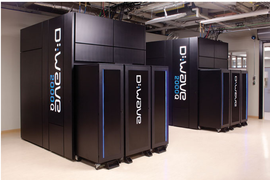
Figure 9.5: The D-Wave 2000Q quantum computer (source: D-Wave).
