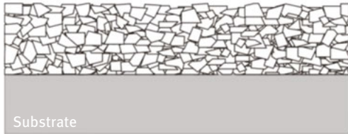
Figure 17.1: Schematic morphology of poly- and nanocrystalline diamond films (left). Scanning electron microscope cross sections of poly- and nanocrystalline diamond films (right).
