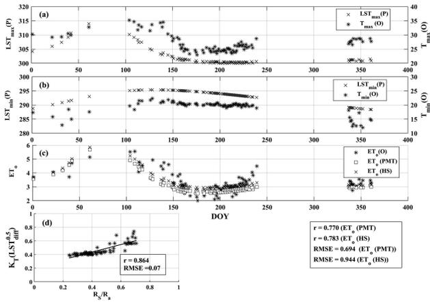
Fig. 7. Comparison of the daily time series of  $LST_{max}$  (K) (a),  $LST_{min}$  (K) (b),  $ET_0$  (mm/day) (c) with ground-based measurements of  $T_{max}$  (°C),  $T_{min}$  (°C), and  $ET_0$  at Berambadi station during 2013 under cloudy sky conditions. Observed  $ET_0$  is estimated using FAO56 PM equation from ground-based measurements. Scatter plot between estimated and observed clearness index (d). Missing data are due to gaps in ground measurements.
