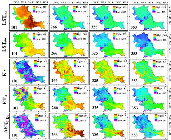
Fig. 9. Spatial variations of  $LST_{max}$  (K),  $LST_{min}$  (K),  $K_v$ ,  $ET_0$  (mm/day), and AET estimated using the vegetation coefficient ( $AET_{VI-K_v}$ ) method (mm/day) for 101st, 266th, 325th, and 353th days of the year 2013, representing different seasons for all-sky conditions.
