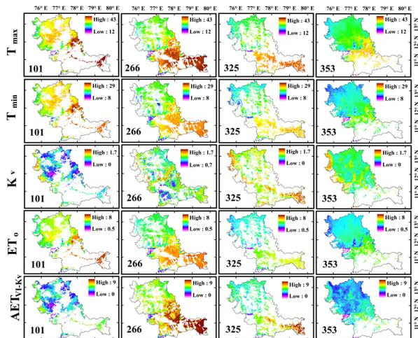
Fig. 5. Spatial variations of  $T_{max}$  ( $^{\circ}C$ ),  $T_{min}$  ( $^{\circ}C$ ),  $K_v$ ,  $ET_0$  (mm/day), and  $ET$  estimated using the vegetation coefficient method ( $AET_{VI-K_v}$ ) (mm/day) for 101st, 266th, 325th, and 353th days of the year 2013, representing different seasons for clear pixels.
