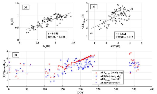
Fig. 8. Scatter plots between  $K_v$  (a),  $AET_{VI-K_v}$  (mm/day) (b) and with their observed values under cloudy sky conditions. Temporal variations of  $AET_{VI-K_v}$  during the year 2013 for all-sky conditions (c). Observed AET values are estimated using Bowen ration technique. Missing data are due to gaps in ground measurements.
